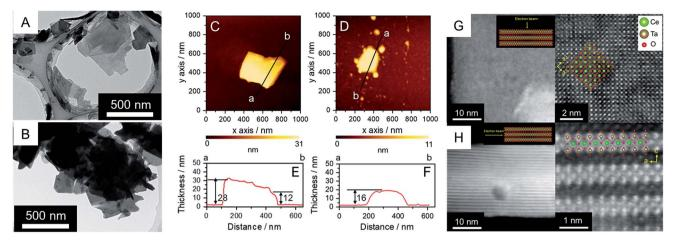
Fig. 2 (A and B) TEM images and (C and D) AFM images with (E and F) thickness profiles for the (A, C and E) anionic TBA- and (B, D and F) chargeneutral Ox-forms. HAADF-STEM images of the Ox-form in the charge-neutral  $[Ce^{iV}Ta_2O_7]$  from (G) basal and (H) vertical views for the layer; (left) lower and (right) higher magnifications.
