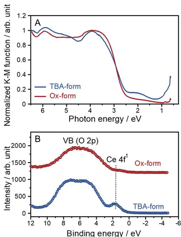
**Fig. 6** (A) Tauc plots and (B) VB XPS spectra for the TBA- and Ox-forms.
