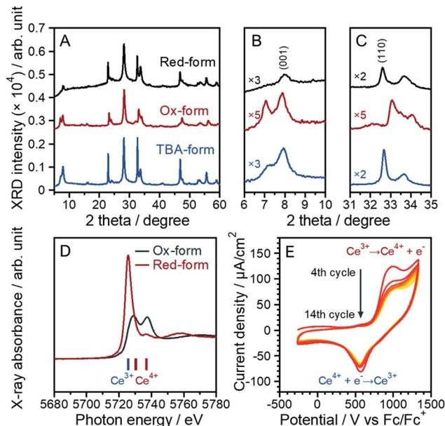
Fig. 8 (A–C) XRD patterns of the TBA-, Ox- and red-forms. (D) Ce  $L_3$ -edge XANES spectra of the Ox- and red-forms. (E) Cyclic voltammograms of the fabricated electrode at a scan rate of  $100 \text{ mV s}^{-1}$ . The CV measurement was conducted in acetonitrile containing 100 mM TBAPF<sub>6</sub>.
