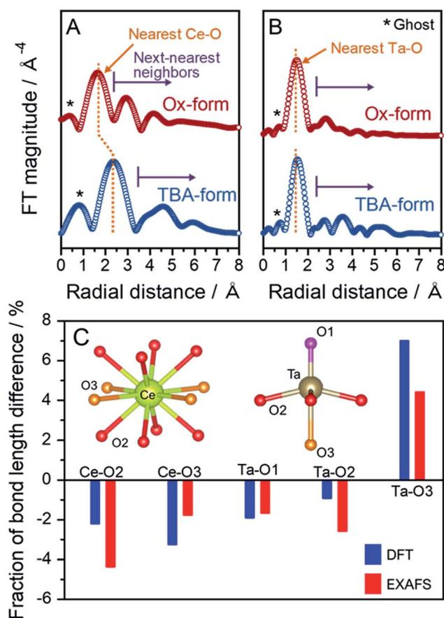
Fig. 5 Fourier transformed (FT) EXAFS spectra in the  $R$ -space at the (A) Ce and (B) Ta  $L_3$ -edges for the TBA- and Ox-forms. (C) Percentages of the bond length changes between the TBA- and Ox-forms obtained from DFT calculations and EXAFS analysis.
