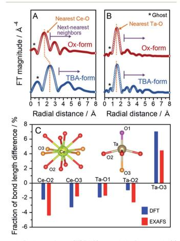
Fig. 5 Fourier transformed (FT) EXAFS spectra in the R-space at the (A) Ce and (B) Ta  $L_3$ -edges for the TBA- and Ox-forms. (C) Percentages of the bond length changes between the TBA- and Ox-forms obtained from DFT calculations and EXAFS analysis.
