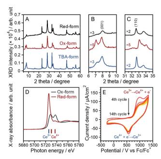
Fig. 8 (A-C) XRD patterns of the TBA-, Ox- and red-forms. (D) Ce  $L_3$ -edge XANES spectra of the Ox- and red-forms. (E) Cyclic voltammograms of the fabricated electrode at a scan rate of 100 mV s $^{-1}$ . The CV measurement was conducted in acetonitrile containing 100 mM TBAPF<sub>6</sub>.
