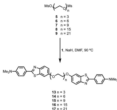
Scheme 2 Synthesis of monodisperse BTA-PEG<sub>n</sub>-BTA dimers.
