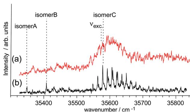
Fig. 11 Action spectrum of the PhOH-(NH<sub>3</sub>)<sub>4</sub> cluster obtained by (a) a ps laser which has a larger band width and (b) a ns laser of higher spectral resolution. The first photon, which is scanned in wavelength, excites the cluster to  $S_1$  and the second photon ionizes the  $\cdot\text{NH}_4(\text{NH}_3)_3$  reaction product. From the IR-UV experiment, three isomers (A, B and C) have been identified.
