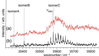
Fig. 11 Action spectrum of the PhOH–(NH<sub>3</sub>)<sub>4</sub> cluster obtained by (a) a ps laser which has a larger band width and (b) a ns laser of higher spectral resolution. The first photon, which is scanned in wavelength, excites the cluster to  $S_1$  and the second photon ionizes the 'NH<sub>4</sub>(NH<sub>3</sub>)<sub>3</sub> reaction product. From the IR-UV experiment, three isomers (A, B and C) have been identified.
