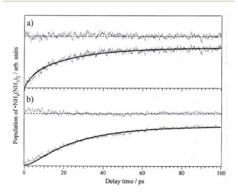
Fig. 10 The time evolutions of the products (a)  ${}^{\circ}NH_4-NH_3-NH_3$  monitored at 12 000 cm $^{-1}$ , (b) the final product  $NH_3-{}^{\circ}NH_4-NH_3$  monitored at 6000 cm $^{-1}$ , for ESHT in the PhOH $-(NH_3)_3$  cluster. The fitted results are shown as solid curves along with the residual. Reproduced from ref. 43 with permission of AIP Publishing, copyright 2007.
