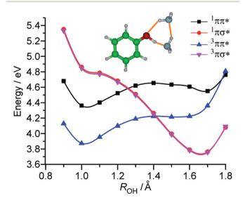
Fig. 7 Potential curves of the PhOH–(NH<sub>3</sub>)<sub>2</sub> cluster along the OH bond length  $R_{\rm OH}$  in different electronic states and spin multiplicities obtained at the RI-CC2/aug-cc-pVDZ level.  $C_{\rm s}$  symmetry has been imposed for the calculations, thus avoided crossing should be considered between  $^{1.3}\pi\pi^*$  and  $^{1.3}\pi\sigma^*$  states. Reproduced from ref. 54 with permission from the PCCP Owner Societies, copyright 2020.
