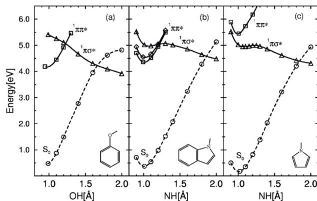
Fig. 4 Potential energy profiles of the lowest <sup>1</sup>ππ\* states (squares), the lowest <sup>1</sup>πσ\* state (triangles) and the electronic ground state (circles) as a function of the OH stretch (PhOH) or NH stretch (indole, pyrrole) reaction coordinate. Geometries have been optimized in the excited electronic states at the CASSCF level; the PE profiles have been obtained with the CASPT2 method. Reproduced from ref. 23 with permission from the PCCP owner Societies, copyright 2002.
