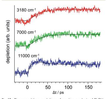
Fig. 13 Picosecond time-evolutions of reaction products of PhOH–(NH $_3$ ) $_4$  measured by the transitions in the IR (NH vibrations at 3180 cm $^{-1}$  (red curve)) and NIR (electronic excitation). Blue curve – excitation at 11 000 cm $^{-1}$  – probes the 'NH $_4$ (NH $_3$ ) $_3$  in the chain structure (4c). Green curve – excitation at 7000 cm $^{-1}$  – probes the most stable  $C_{3v}$  structure (4a): this structure is obtained at longer delay times.
