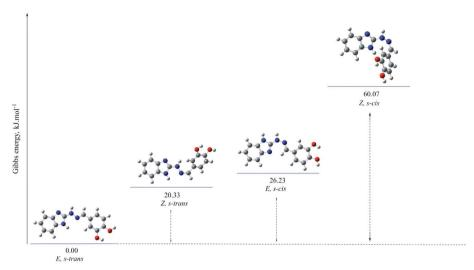
Fig. 4 Optimized molecular structure and relative Gibbs energies (in kJ  $mol^{-1}$ ) of the possible isomers of compound 5d in amino tautomeric form, obtained at B3LYP/6-311++G(d,p) level of theory in gas phase.
