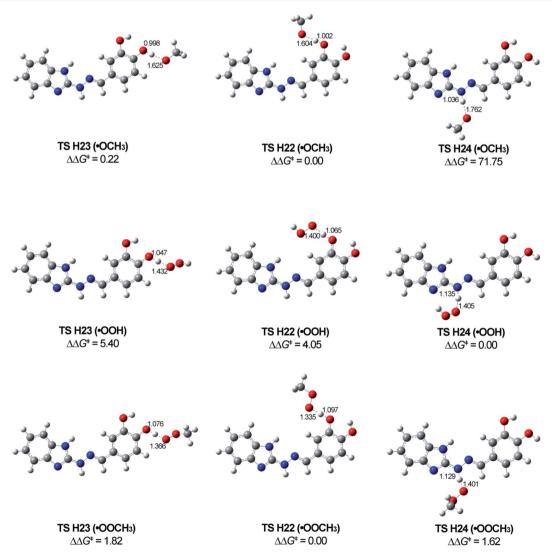
Fig. 9 Optimized structures of the TSs for the most stable radicals R2, R3 and R4 corresponding to the HAT mechanism.  $\Delta\Delta G^{\ddagger}$  shows the difference in the activation energies between the TSs for every one of the studied radicals. Calculations are done on SP M06-2X/6-311++G\*\* method in solvent water.
