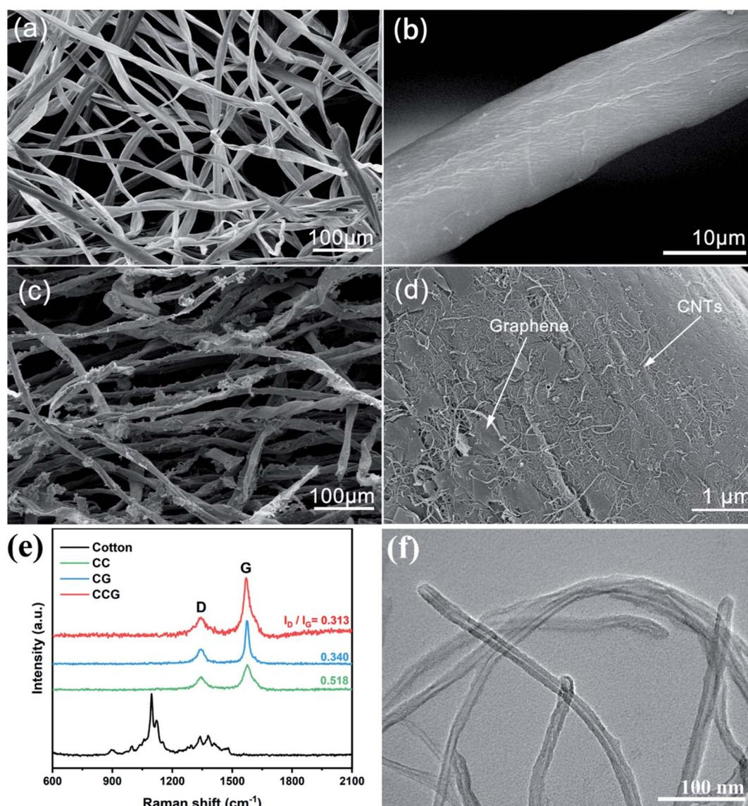
Fig. 2 SEM images of (a and b) cotton fibers, (c and d) CCG substrates. (e) Raman spectra of cotton, CC, CG, and CCG substrates. (f) High-resolution transmission electron microscope (HRTEM) image of CNTs.
