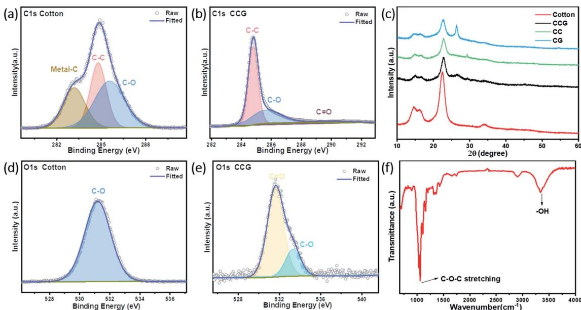
Fig. 3 Carbon 1s XPS spectra of (a) cotton fibers and (b) CCG substrate. (c) XRD patterns of cotton, CC, CG, and CCG substrates. Oxygen 1s XPS spectra of (d) cotton fibers and (e) CCG substrate. (f) FTIR spectra of the cotton fiber.
