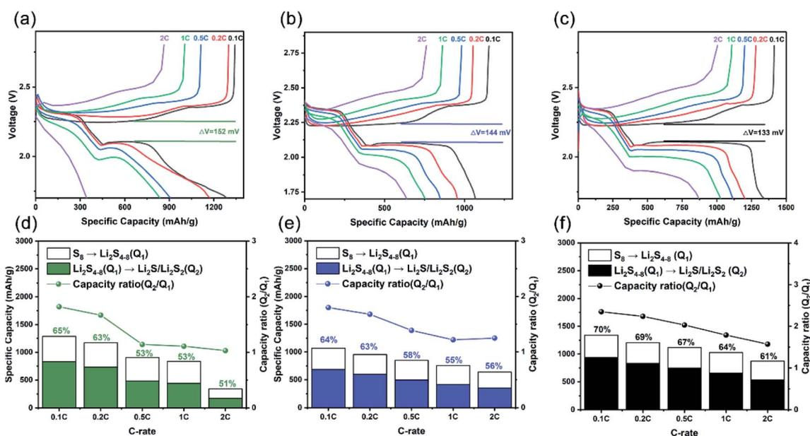
Fig. 5 Charge and discharge specific capacity versus voltage profiles of the (a) CC, (b) CG, (c) CCG substrate batteries from 0.1C to 2C. Capacity contribution of lower potential ( $Q_1$ ) and higher potential ( $Q_2$ ) and the  $Q_2/Q_1$  ratio at various C rates for the (d) CC, (e) CG, (f) CCG substrate batteries.
