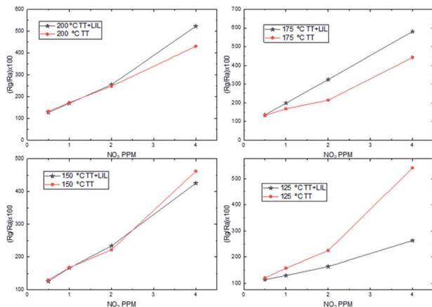
Fig. 4 Dynamic response curves of zinc oxide (only annealed and processed with laser interference) to decreasing  $\text{NO}_2$  concentrations (4, 2, 1 and 0.5 ppm) at 4 different temperatures (200 to 125 °C).
