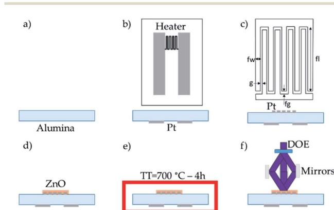
**Fig. 1** (a) Cross section of the alumina substrate. (b) Cross section and top view of the platinum deposited to perform as a heater. (c) Cross section and top view of interdigitated electrodes. (d) ZnO deposited on the interdigitated electrodes. (e) Thermal treatment (TT) of the ZnO deposited at 700 °C for 4 h. (f) ZnO structuration by LIL.
