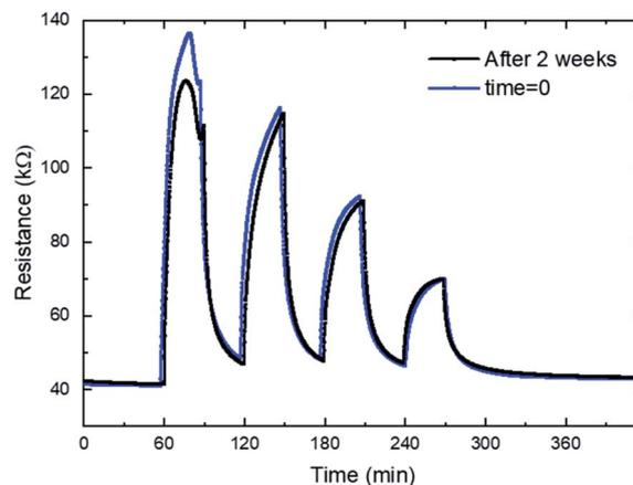
**Fig. 8** Dynamic response curves of zinc oxide (only annealed) to decreasing NO<sub>2</sub> concentrations (4, 2, 1 and 0.5 ppm) at 200 °C for a new gas sensor and after two weeks.
