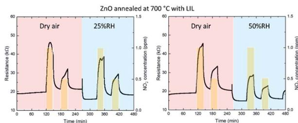
Fig. 10 Dynamic response curves of zinc oxide (after annealing and LIL) to decreasing  $\text{NO}_2$  concentrations (1 and 0.5 ppm) at 200 °C with dry air and 25% or 50% of relative humidity conditions.
