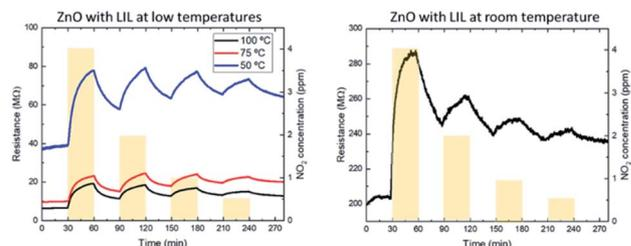
Fig. 6 Dynamic response curves of zinc oxide (only annealed and processed with laser interference) to decreasing  $\text{NO}_2$  concentrations (0.5 to 4 ppm range) at 3 different temperatures (100, 75 and 50 °C) (left) and at room temperature (right).
