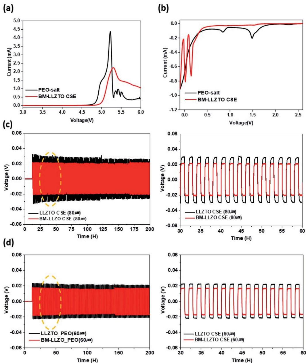
Fig. 5 LSV curves of the PEO salt and BM-LLZTO CSE over the oxidation reaction range (a) and the reduction reaction range (b). Li/CSEs/Li symmetric cell voltage profiles for CSEs with 80  $\mu\text{m}$  (c) and 60  $\mu\text{m}$  (d) thickness at 0.1  $\text{mA cm}^{-2}$ .
