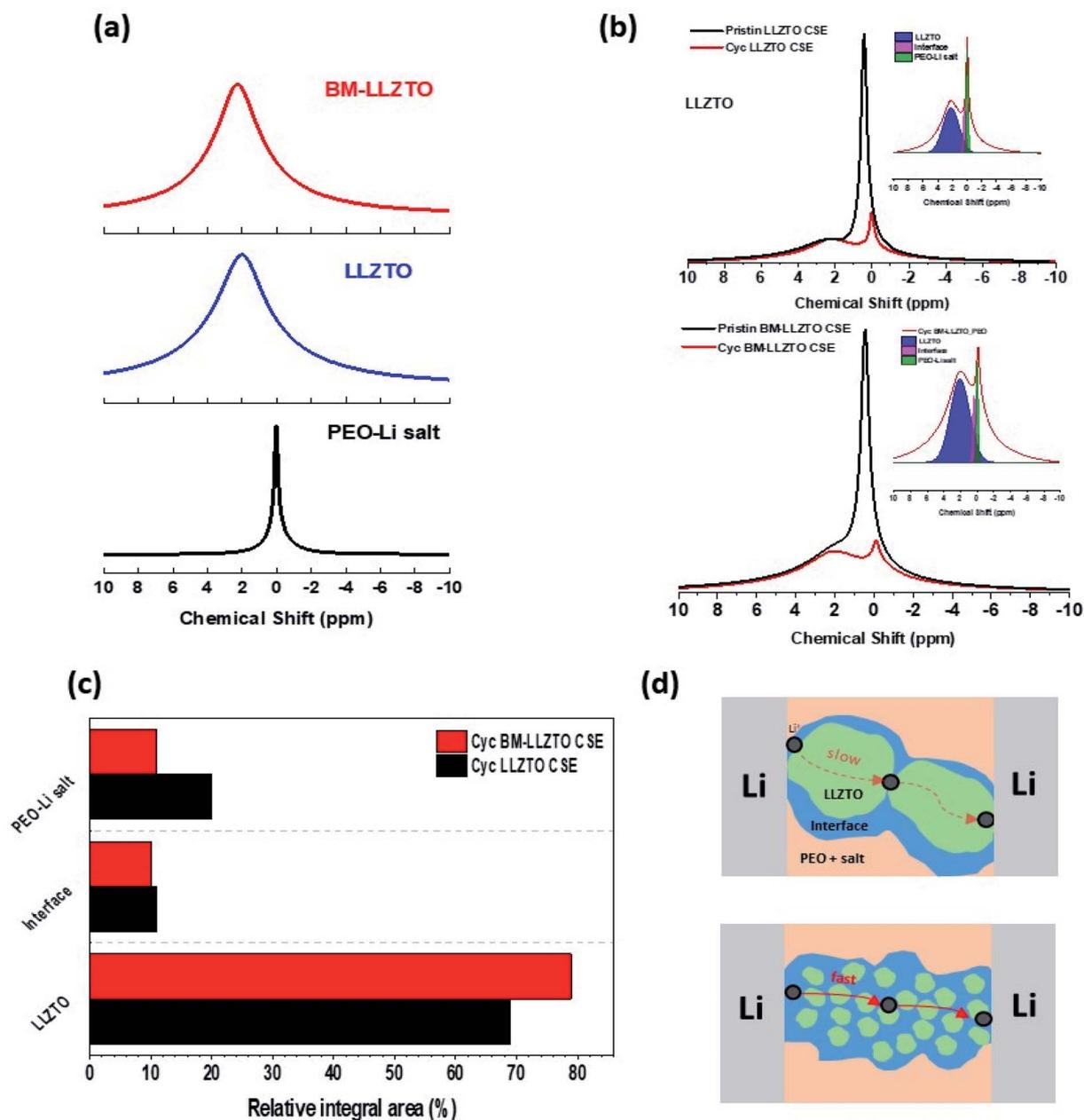
Fig. 4 MAS  $^7\text{Li}$  NMR spectra of PEO-Li salt, LLZTO, and BM-LLZTO (a);  $^7\text{Li}$  NMR profiles of the pristine CSE and the CSE after cycling in a  $^6\text{Li}/\text{CSEs}/^6\text{Li}$  symmetric cell (b); the calculated relative integral area value exhibited by the CSE after cycling (c); schematic diagram of the Li-ion transport mechanism exhibited by the CSEs according to their particle size.
