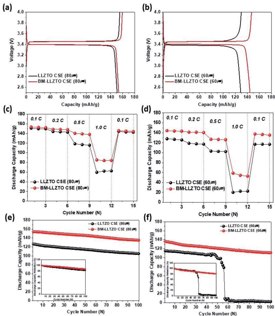
Fig. 6 0.1C initial charge/discharge curve for the CSE having 80  $\mu\text{m}$  (a) and 60  $\mu\text{m}$  (b) thickness; rate capacity determined at various current densities between 0.1 and 1.0C at 80  $\mu\text{m}$  (c) and 60  $\mu\text{m}$  (d) thickness; cycling performance at 0.33C for CSEs with 80  $\mu\text{m}$  (e) and 60  $\mu\text{m}$  (f) thickness.
