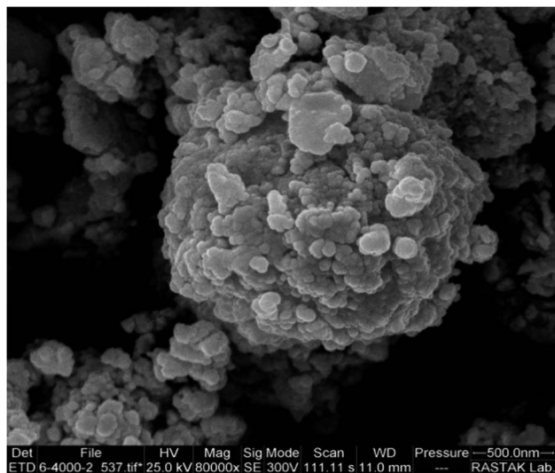
Fig. 8 SEM image of Cu-TBA@biochar nanoparticles. Adapted with consent from ref. 74. Copyright Elsevier.
