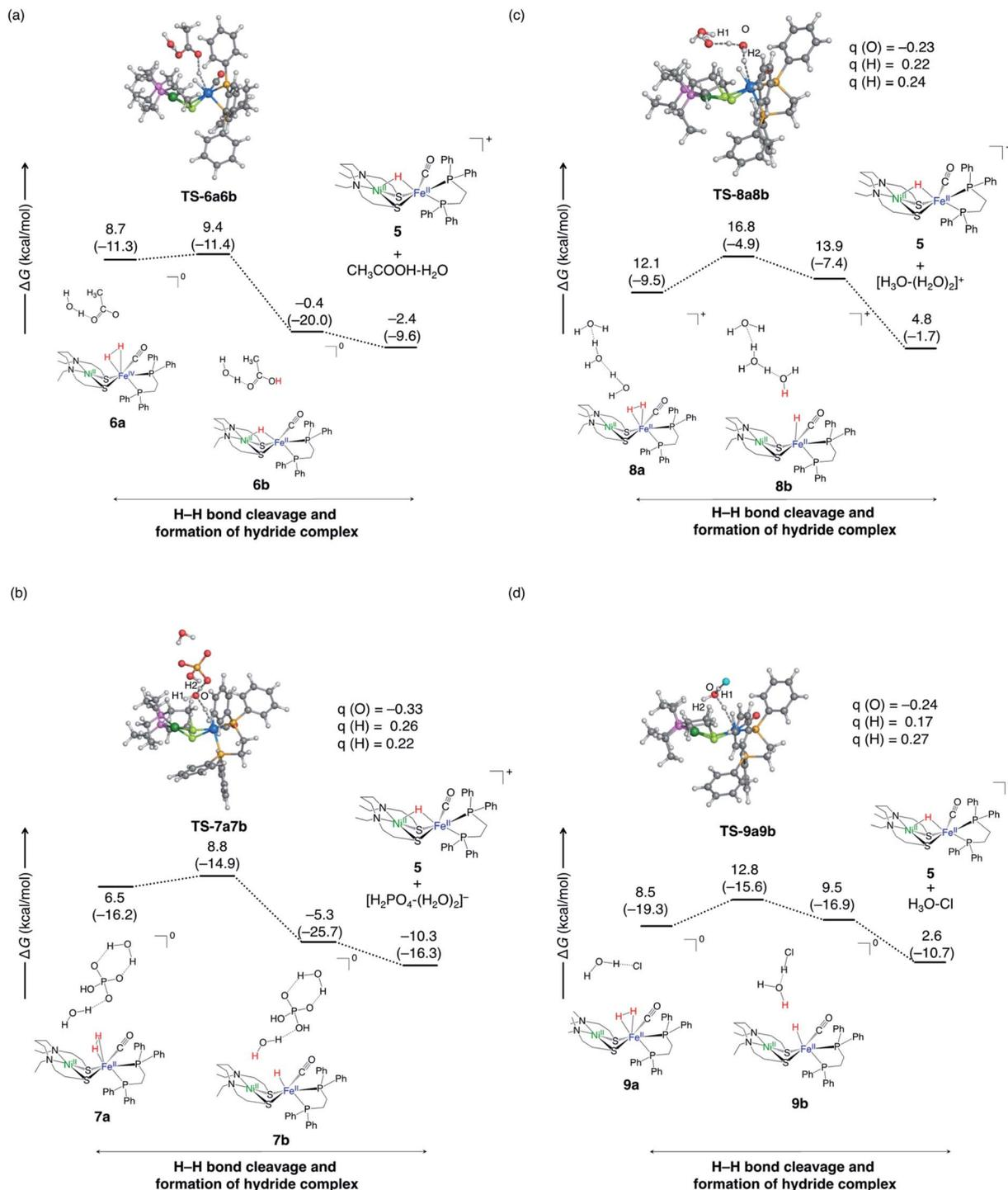
Fig. 10 Free energy profiles of proton abstraction by Lewis base from NiFe dihydrogen complex for four reactions; (a) for (R3), (b) for (R4), (c) for (R5), and (d) for (R6).  $\Delta G$  and  $\Delta H$  values (in parentheses) are in  $\text{kcal mol}^{-1}$ . The selected atomic charges,  $q$ , are also shown.
