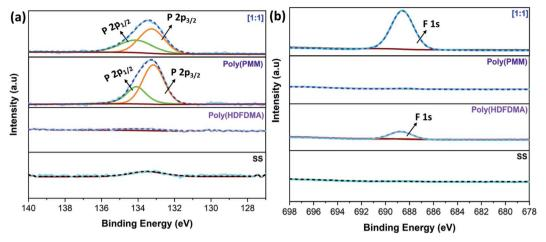
Fig. 8 (a) XPS core-level high resolution P 2p scans, and (b) F 1s scans, for uncoated, poly(HDFDMA) homopolymer coated, poly(HDFDMA-co-PMM) copolymer with mol ratio [1:1] coated SS coupon surfaces.
