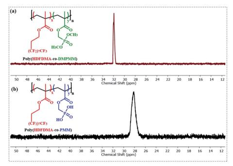
Fig. 3 (a)  $^{31}P$  NMR (400 MHz) spectra of poly(HDFDMA-co-DMPMM) protected copolymer, and (b) the resulting hydrolyzed (deprotected) poly(HDFDMA-co-PMM) copolymer for mol ratio [1 : 1]. Both spectra were taken in deuterated trifluoroacetic acid (CF<sub>3</sub>CO<sub>2</sub>D).
