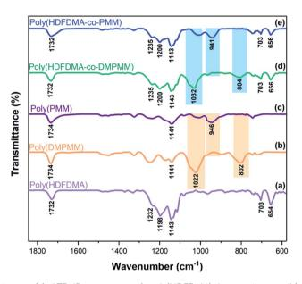
Fig. 4 (a) ATR-IR spectrum of poly(HDFDMA) homopolymer, (b) protected poly(DMPMM) homopolymer, (c) deprotected poly(PMM) homopolymer, (d) protected poly(HDFDMA-co-DMPMM) copolymer [1:1], and (e) deprotected poly(HDFDMA-co-PMM) copolymer [1:1].
