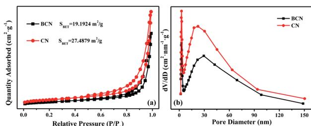
**Fig. 4** (a) N<sub>2</sub> adsorption-desorption isotherm, (b) aperture distribution and curve of BCN and CN.
