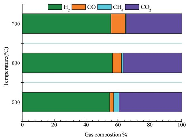
Fig. 9 Gas composition of acetic acid steam reforming over Ni/SiO<sub>2</sub>.
