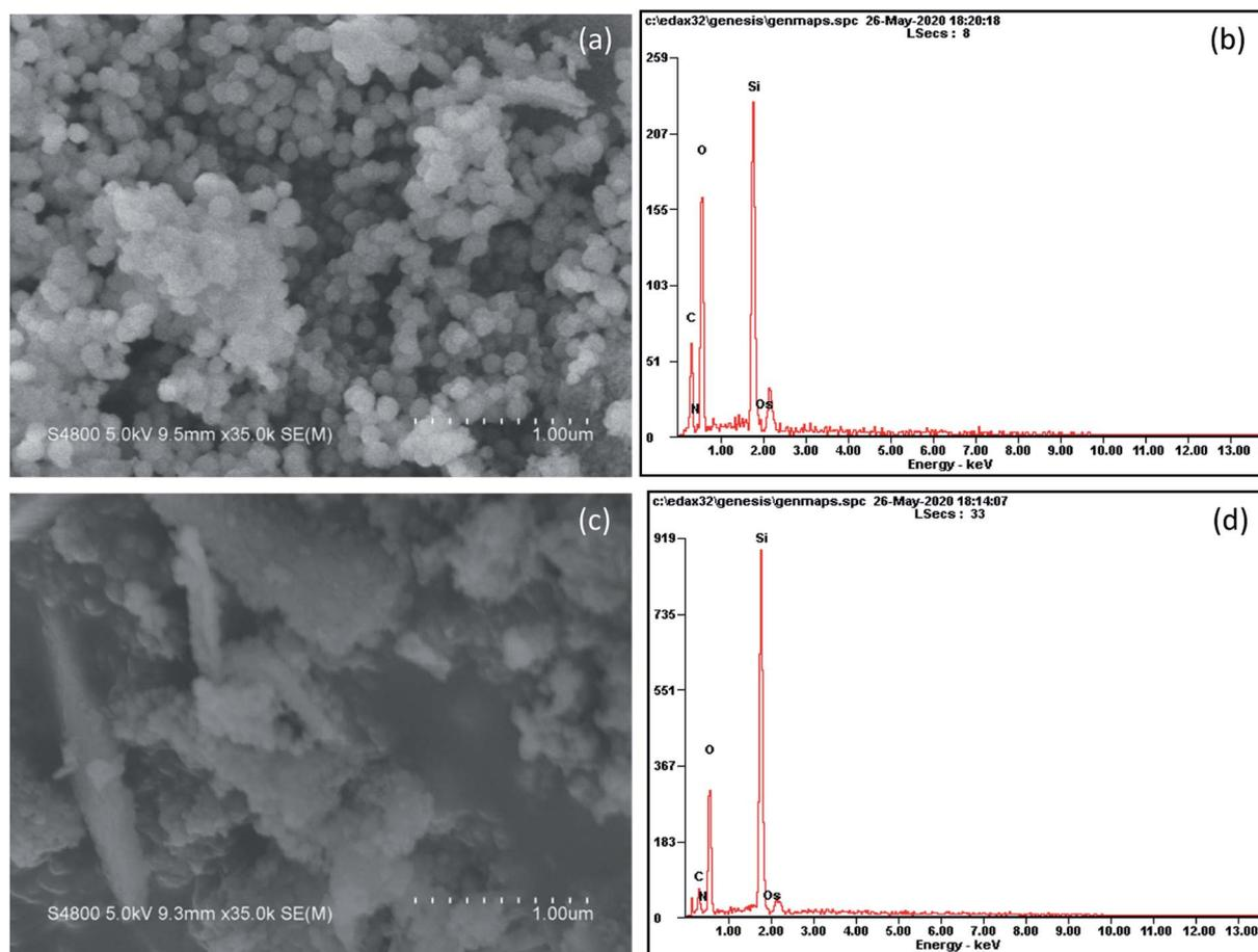
Fig. 4 The morphology of samples pyrolyzed at (a and b) 500 °C and (c and d) 700 °C.
