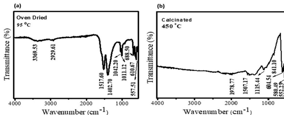
Fig. 1 FTIR analysis of *A. viridis*-assisted CuO–Bi<sub>2</sub>O<sub>3</sub> nanocomposite. (a) FTIR spectrum of dried material at 95 °C. (b) FTIR spectrum of thermally treated material at 450 °C.
