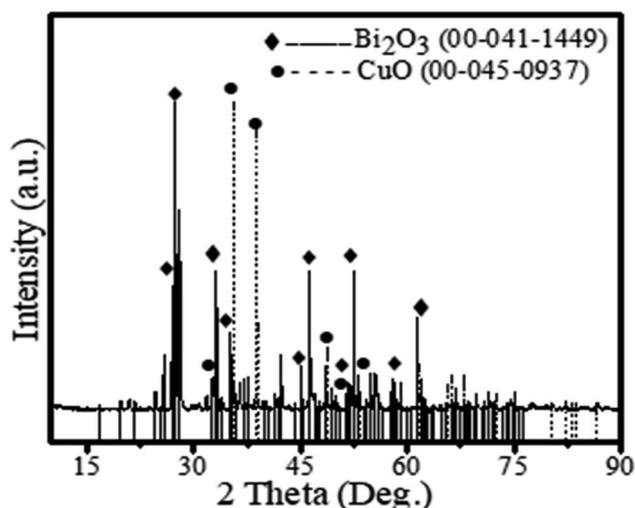
Fig. 2 XRD patterns of the AVL-mediated CuO–Bi<sub>2</sub>O<sub>3</sub> nanocomposite.
