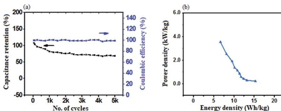
Fig. 7 (a) Capacitance retention and coulombic efficiency (%) of the CuO–Bi<sub>2</sub>O<sub>3</sub> electrode, demonstrating the stability of the electrode. (b) Ragone plot of the fabricated CuO–Bi<sub>2</sub>O<sub>3</sub> electrode.
