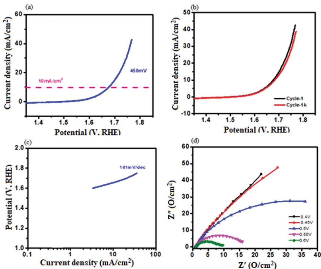
Fig. 9 OER measurements. (a) Polarization curve. (b) Cycling runs of the CuO–Bi<sub>2</sub>O<sub>3</sub> nanocomposite by LSV. (c) Tafel slope. (d) Variation of impedance as a function of frequency at various overpotentials.
