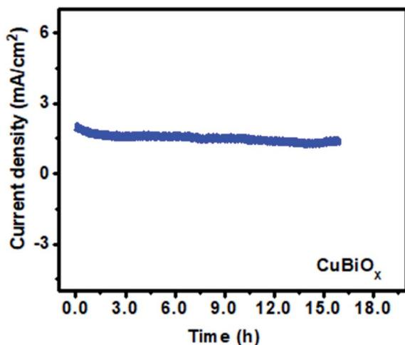
Fig. 10 Stability test of CuO–Bi<sub>2</sub>O<sub>3</sub> for overall water splitting.
