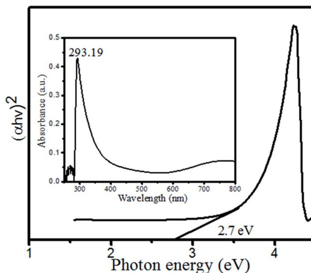
Fig. 5 Tauc plot of the CuO–Bi<sub>2</sub>O<sub>3</sub> nanocomposite: inset (UV-visible spectrum of CuO–Bi<sub>2</sub>O<sub>3</sub>).
