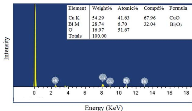
Fig. 3 EDX analysis for elemental composition of the CuO–Bi<sub>2</sub>O<sub>3</sub> nanocomposite.
