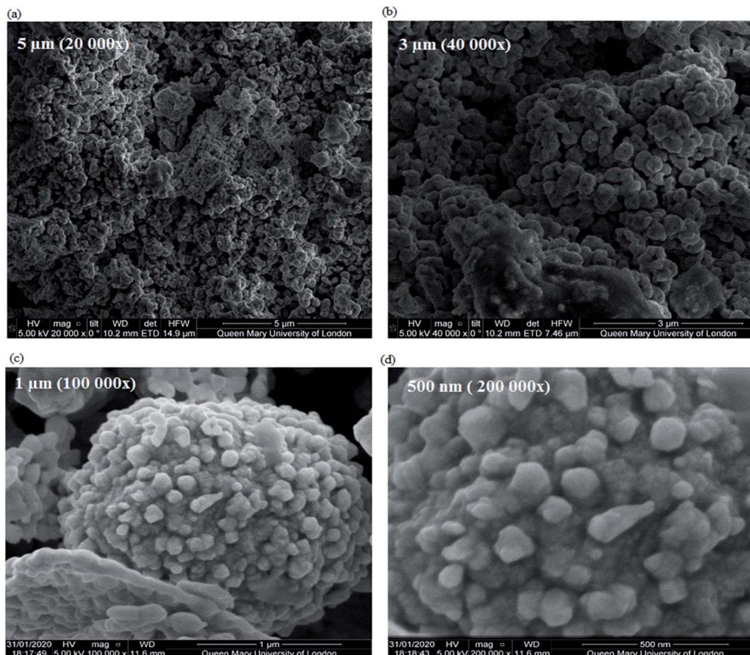
Fig. 4 FE-SEM images of CuO–Bi<sub>2</sub>O<sub>3</sub> nanocomposites at (a) 5 μm, (b) 3 μm, (c) 1 μm, and (d) 500 nm.
