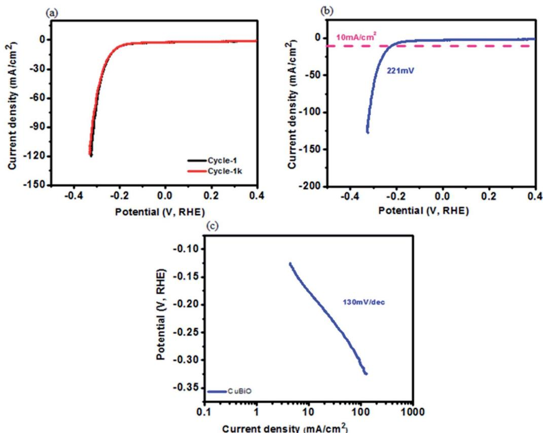
Fig. 8 HER measurements. (a) Cyclic stability of the CuO–Bi<sub>2</sub>O<sub>3</sub> nanocomposite by LSV. (b) Polarization curve of the CuO–Bi<sub>2</sub>O<sub>3</sub> nanocomposite. (c) Tafel slope of the CuO–Bi<sub>2</sub>O<sub>3</sub> nanocomposite.
