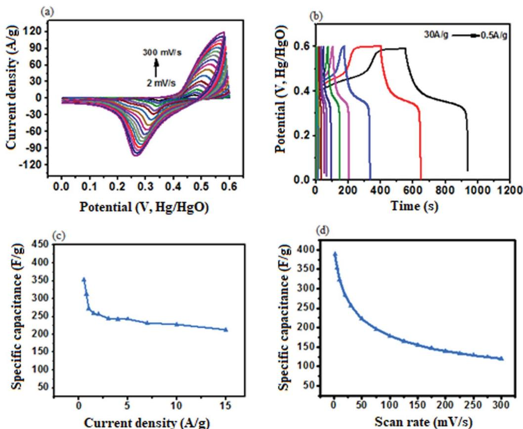
Fig. 6 (a) CV profile of CuO–Bi<sub>2</sub>O<sub>3</sub>. (b) GCD measurements of CuO–Bi<sub>2</sub>O<sub>3</sub>. (c) Calculated specific capacity at different current densities. (d) Calculated specific capacity at different scan rates.
