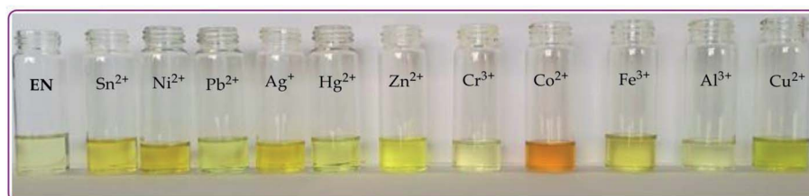
Fig. 2 Observable colorimetric changes of the cations (0.03 M) upon interacting with EN ( 1 \times 10^{-5} M) in DMSO–H 2 O at room temperature.
