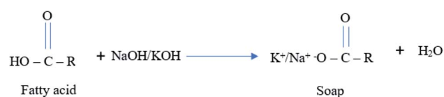
Fig. 5 Soap formation during alkaline catalytic transesterification of non-edible oil containing excessive amount of FFAs.
