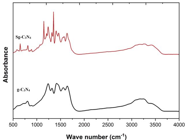
Fig. 6 FT-IR spectra of g-C<sub>3</sub>N<sub>4</sub> and Sg-C<sub>3</sub>N<sub>4</sub>.
