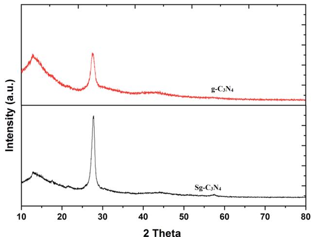
Fig. 2 XRD patterns of g-C<sub>3</sub>N<sub>4</sub> and Sg-C<sub>3</sub>N<sub>4</sub>.
