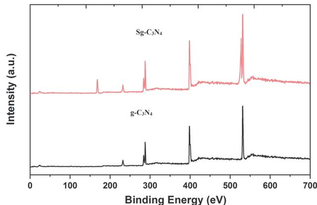
Fig. 8 XPS survey scans of g-C<sub>3</sub>N<sub>4</sub> and Sg-C<sub>3</sub>N<sub>4</sub>.
