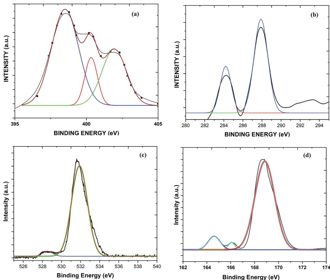
Fig. 7 XPS spectra: (a) the N 1s spectrum of Sg-C<sub>3</sub>N<sub>4</sub>, (b) the C 1s spectrum of Sg-C<sub>3</sub>N<sub>4</sub>, (c) the O 1s spectrum of Sg-C<sub>3</sub>N<sub>4</sub>, and the (d) S 2p spectrum of Sg-C<sub>3</sub>N<sub>4</sub>.
