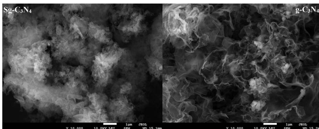
Fig. 3 SEM images of Sg-C<sub>3</sub>N<sub>4</sub> and g-C<sub>3</sub>N<sub>4</sub>.
