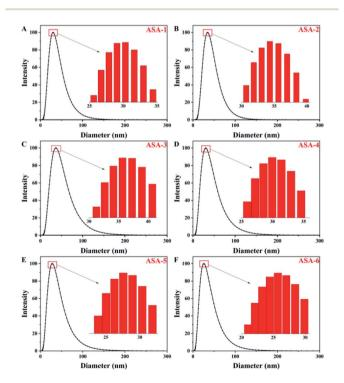
Fig. 4 Particle-size distributions of the PBA latex particles: (A) ASA-1, (B) ASA-2, (C) ASA-3, (D) ASA-4, (E) ASA-5, and (F) ASA-6.
