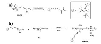
Fig. 1 Synthetic pathway for preparing Si-PBA.
