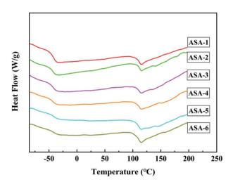
Fig. 7 DSC curves of ASA powders.
