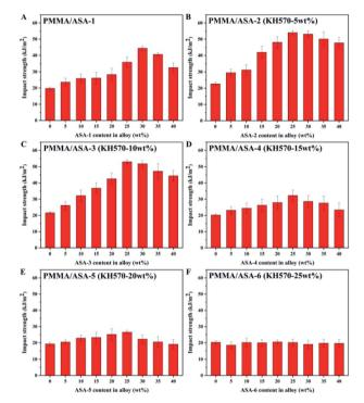
Fig. 9 Impact strengths of the PMMA/ASA alloys.
