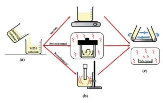
Fig. 2 Representation of the process of ZIF-8 formation: (a) solution preparation, (b) crystallization, (c) washing and activation method.
