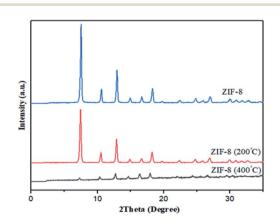
Fig. 6 XRD patterns of heated ZIF-8 at 200, 400 °C.
