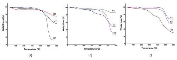
Fig. 5 TGA curves of the synthesized ZIF-8 in different solvents. (a) Mixing method, (b) solvothermal method, (c) sonochemical method.
