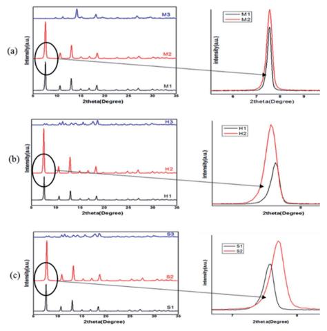
Fig. 3 XRD patterns of ZIF-8 samples synthesized with different solvents (water, MeOH, DMF) at different conditions: (a) mixing method, (b) solvothermal method. (c) ultrasonic method.
