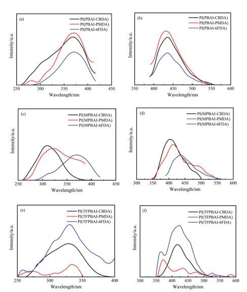
Fig. 12 Excitation – emission spectra of polyimide solution in DMAc  $(1 \times 10^{-4} \text{ g L}^{-1})$  (a) excitation spectra of PIs with PBAI, (b) emission spectra of Pls with PBAI, (c) excitation spectra of Pls with MPBAI (d) emission spectra of Pls with MPBAI, (e) excitation spectra of Pls with TFPBAI, (f) emission spectra of PIs with TFPBAI
