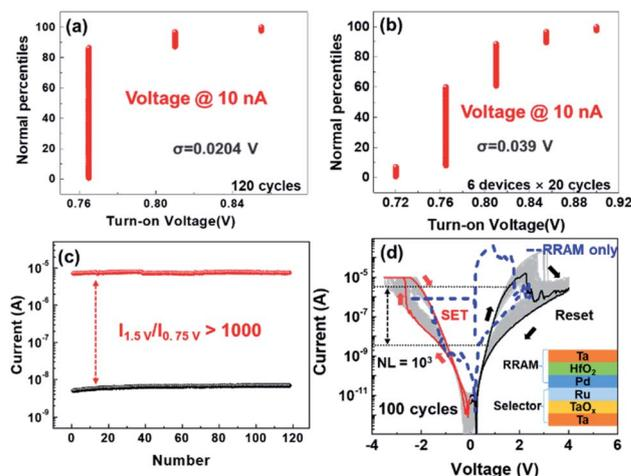
Fig. 2 (a) Cumulative probability of the turn-on voltage for 120 cycles. (b) Cumulative probability of the turn-on voltage for 6 different devices with 20 cycles. (c) The current at  $V_{read}$  (1.5 V) and  $1/2V_{read}$  (0.75 V) for 120 cycles. (d)  $I$ - $V$  curves of the 1S1R cell for 100 cycles. (Inset: the structure of 1S1R cell.)
