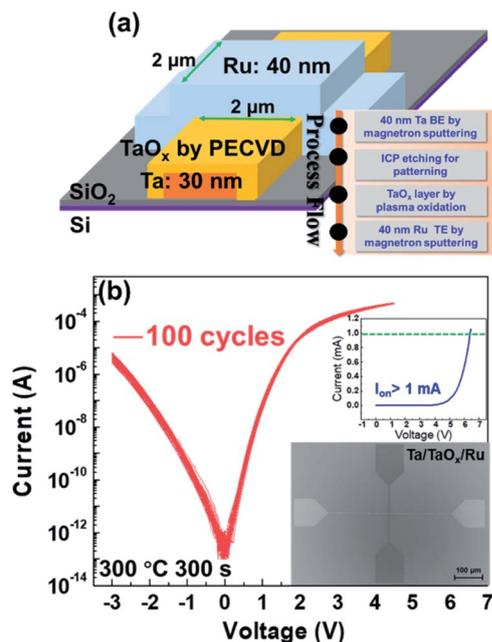
Fig. 1 (a) Schematic diagram of the devices and the process flow of the devices. (b)  $I$ - $V$  characteristics of the Ta/TaO<sub>x</sub>/Ru device as selector plotted in semi-log scale and linear scale (inset). Inset: SEM image of the Ta/TaO<sub>x</sub>/Ru device. (Oxidation parameters: 300 °C, 300 s.)
