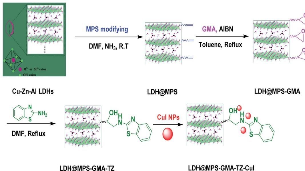
Scheme 1 Schematic representation for preparation of LDH@MPS-GMA-TZ-CuI nanocomposite.
