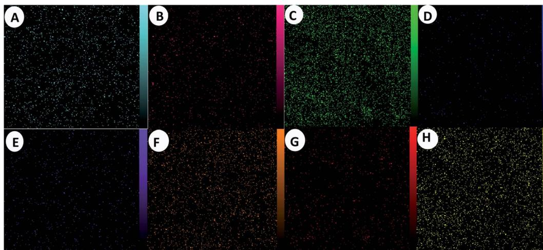
Fig. 4 Elemental mapping of the A (Zn), B (S), C (O), D (N), E (I), F (Cu), G (C), H (Al) atoms achieved from SEM micrographs.
