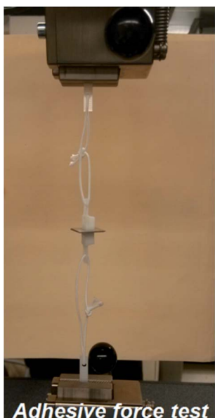
Fig. 4 Test method of adhesive performance of the SMPS microparticles using a universal testing machine.
