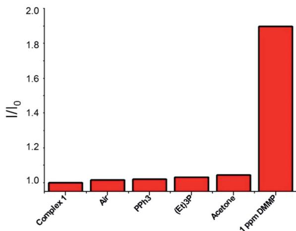
Fig. 3 Selectivity tests: normalized fluorescence responses of complex **1** ( $1 \times 10^{-6} \text{ M}$  in chloroform,  $\lambda_{\text{ex}} 422 \text{ nm}$ ) towards air (bubbled for 5 min),  $\text{PPh}_3$  (2 ppm),  $(\text{Et})_3\text{P}$  (2 ppm), acetone (2 ppm), and **DMMP** (1 ppm). Analytes are sequentially added up to the final addition of **DMMP**. Bars represent the final ( $I$ ) over the initial ( $I_0$ ) emission intensity at 625 nm.
