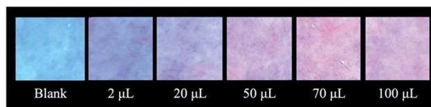
Fig. 4 Qualitative tests of complex **1** absorbed onto the filtration paper and exposed to an increasing amount of **DMMP** vapours ( $2 \mu\text{L}$ ,  $20 \mu\text{L}$ ,  $50 \mu\text{L}$ ,  $70 \mu\text{L}$ ,  $100 \mu\text{L}$ , at  $60 \text{ }^\circ\text{C}$ ).
