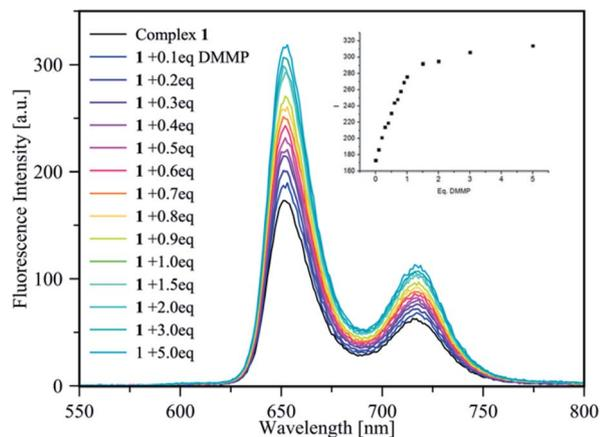
Fig. 2 Fluorescence titration of complex **1** ( $1 \mu\text{M}$  in  $\text{CHCl}_3$ ) with increasing amount of **DMMP** (0–5 eq.); the inset shows the intensity increase upon the progressive addition of **DMMP** equivalents.
