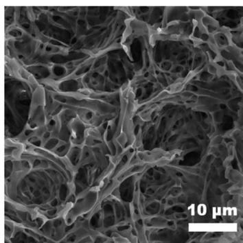
Fig. 9 High-magnification SEM image of the coating layers formed by N-50 (5 mL, 10 mg mL<sup>-1</sup>) with 2 μL water.
