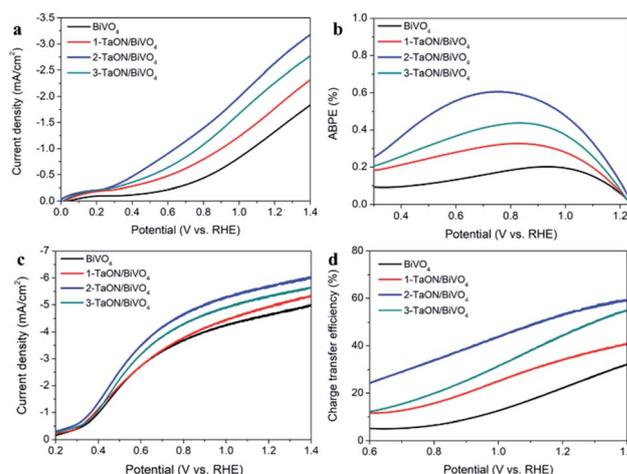
Fig. 3 (a) LSV curves in the PBS solution, (b) ABPE values, (c) LSV curves in the PBS solution containing 0.1 M  $\text{Na}_2\text{SO}_3$  and (d) the charge transfer efficiencies of different electrodes.
