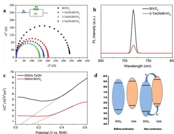
Fig. 4 (a) Electrochemical impedance spectroscopy (EIS) of different electrodes. (b) PL measurements of the BiVO<sub>4</sub> and 2-TaON/BiVO<sub>4</sub> electrode (exciting source: 360 nm). (c) The Mott-Schottky plots of BiVO<sub>4</sub> and TaON. (d) The charge transfer mechanism of the TaON/BiVO<sub>4</sub> electrode.
