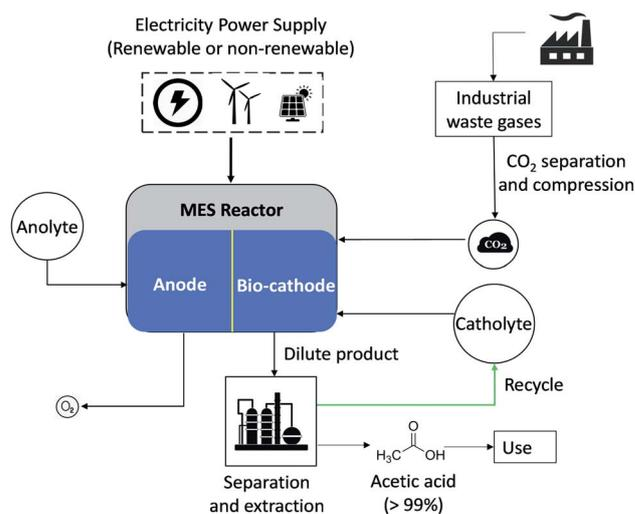
Fig. 1 Schematic representation of AA production in MES reactor system where energy is supplied from either renewable or non-renewable sources and  $\text{CO}_2$  is separated from industrial waste gases.
