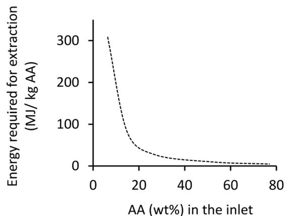
Fig. 3 Energy consumption in extractive distillation as a function of inlet feed concentration of AA.
