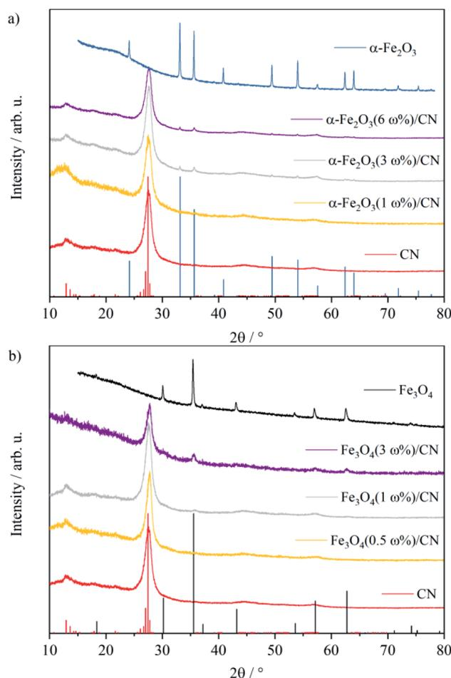
Fig. 2 PXRD patterns of the as-prepared catalysts (a)  $\alpha\text{-Fe}_2\text{O}_3/\text{CN}$  composites,  $\alpha\text{-Fe}_2\text{O}_3$  and (b)  $\text{Fe}_3\text{O}_4/\text{CN}$  composites and  $\text{Fe}_3\text{O}_4$  (references: CN ICDD 00-066-0813,<sup>40</sup> red bars;  $\alpha\text{-Fe}_2\text{O}_3$  ICDD 01-089-0597,<sup>42</sup> blue bars;  $\text{Fe}_3\text{O}_4$  ICDD 00-019-0629,<sup>41</sup> black bars).
