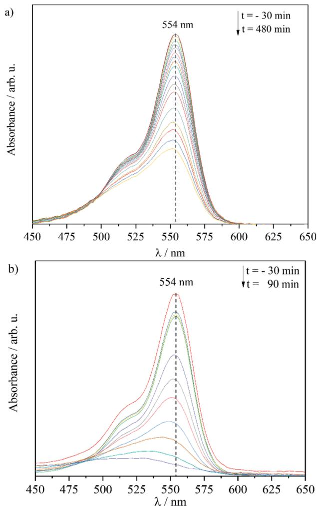
Fig. 8 Visible light spectra of RhB while photodegradation process using (a)  $\alpha\text{-Fe}_2\text{O}_3(3\ \omega\%)/\text{CN-2}$  and (b)  $\alpha\text{-Fe}_2\text{O}_3(3\ \omega\%)/\text{CN}$  particles as photocatalyst.
