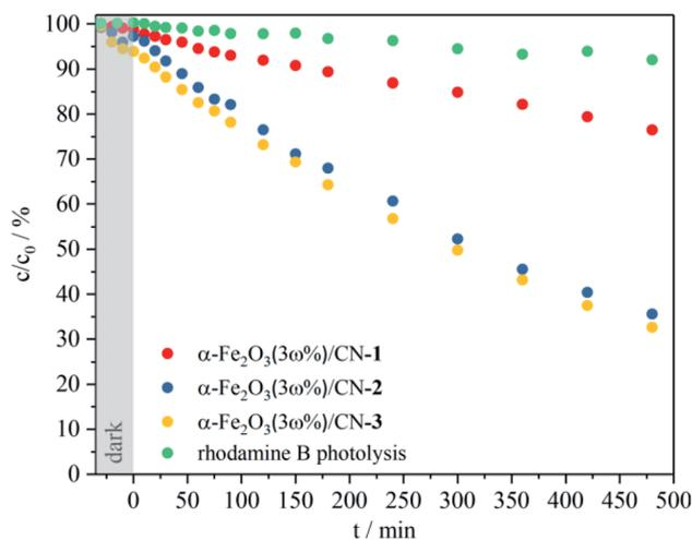
Fig. 7 Time-dependent photodegradation of an aqueous RhB solution ( $1 \times 10^{-5}$  M) under visible light irradiation ( $t > 0$  min) without catalyst and in the presence of coatings  $\alpha\text{-Fe}_2\text{O}_3(3\ \omega\%)/\text{CN-1}$ ,  $\alpha\text{-Fe}_2\text{O}_3(3\ \omega\%)/\text{CN-2}$  and  $\alpha\text{-Fe}_2\text{O}_3(3\ \omega\%)/\text{CN-3}$ .
