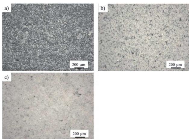
Fig. 6 Light microscope images of coatings with different deposited masses (a)  $\alpha\text{-Fe}_2\text{O}_3(3\ \omega\%)/\text{CN-1}$ , (b)  $\alpha\text{-Fe}_2\text{O}_3(3\ \omega\%)/\text{CN-2}$  and (c)  $\alpha\text{-Fe}_2\text{O}_3(3\ \omega\%)/\text{CN-3}$ , 5 $\times$  magnification.
