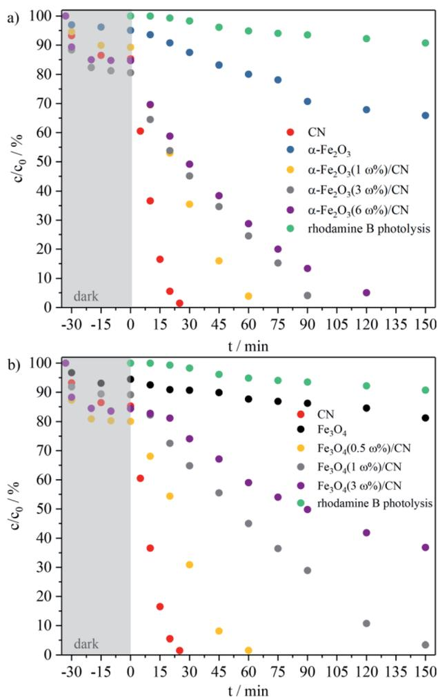
Fig. 5 Time-dependent photodegradation of an aqueous RhB solution ( $1 \times 10^{-5} \text{ M}$ ) under visible light irradiation ( $t > 0 \text{ min}$ ) without catalyst and in the presence of 40 mg  $\alpha\text{-Fe}_2\text{O}_3$ ,  $\text{Fe}_3\text{O}_4$  or CN. (a)  $\alpha\text{-Fe}_2\text{O}_3/\text{CN}$  compounds and (b)  $\text{Fe}_3\text{O}_4/\text{CN}$  compounds as dispersion.
