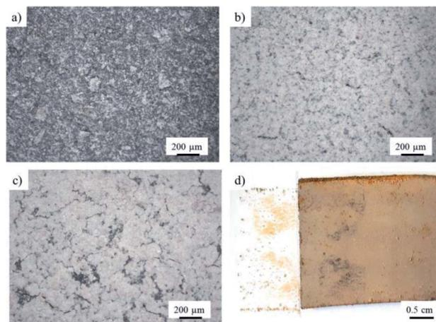
Fig. 9 Light microscope images after catalysis using coatings with different deposited masses (a)  $\alpha\text{-Fe}_2\text{O}_3(3\ \omega\%)/\text{CN-1}$ , (b)  $\alpha\text{-Fe}_2\text{O}_3(3\ \omega\%)/\text{CN-2}$  and (c)  $\alpha\text{-Fe}_2\text{O}_3(3\ \omega\%)/\text{CN-3}$ , 5 $\times$  magnification (d) scotch tape test of sample  $\text{Fe}_2\text{O}_3(3\ \omega\%)/\text{CN-2}$ .
