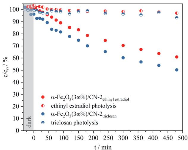
Fig. 10 Time-dependent photodegradation of aqueous ethinyl estradiol and triclosan solutions ( $4 \times 10^{-5}\ \text{M}$ ) under visible-light irradiation ( $t > 0\ \text{min}$ ) without catalyst and in the presence of  $\alpha\text{-Fe}_2\text{O}_3(3\ \omega\%)/\text{CN-2}$  as photocatalytic coating.
