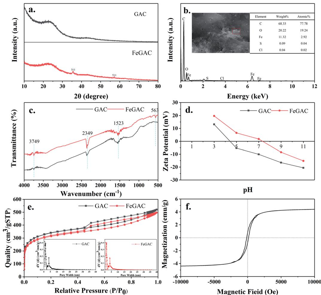
Fig. 2 (a) The XRD profiles of GAC and FeGAC; (b) FeGAC morphology and element compositions; (c) the FTIR spectra of GAC and FeGAC; (d)  $pH_{PZC}$  values of GAC and FeGAC; (e) nitrogen adsorption–desorption isotherm of GAC and FeGAC; (f) VSM plots of FeGAC.
