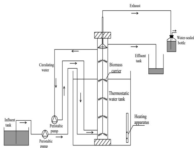
Fig. 1 Schematic diagram of the identical anammox reactor.
