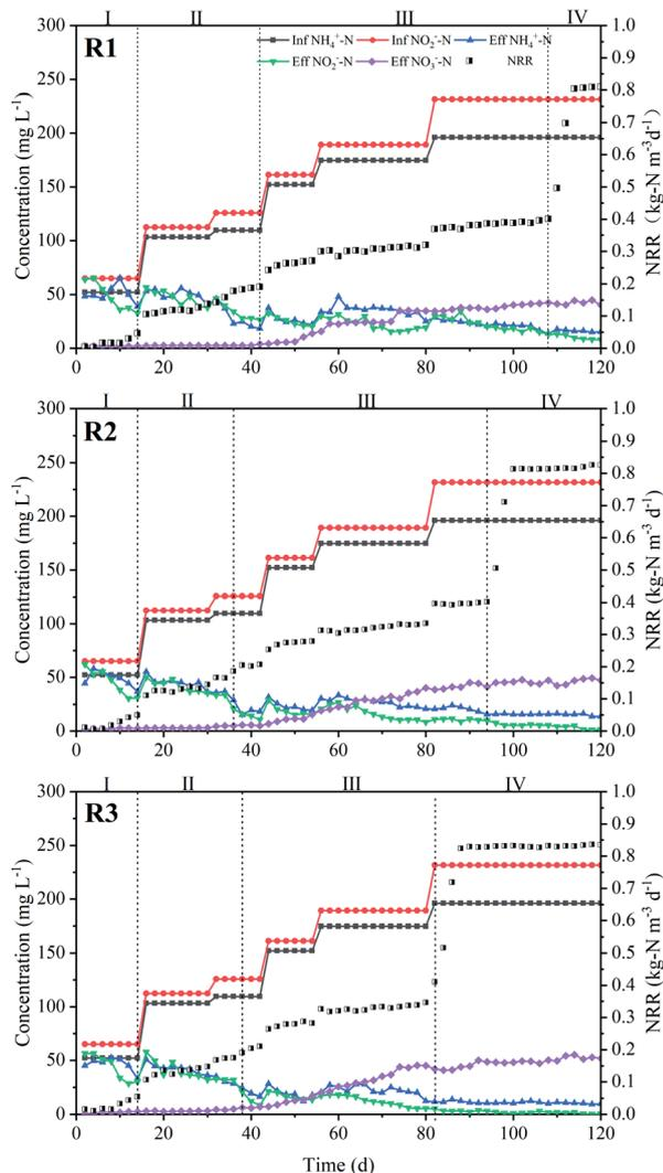
Fig. 3 Nitrogen removal performance of reactors during start-up period.
