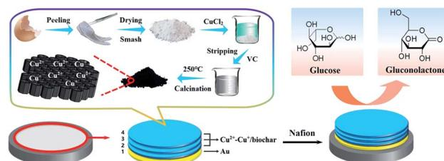
Scheme 1 The fabrication process of the nonenzyme glucose sensing based Cu<sup>2+</sup>–Cu<sup>+</sup>/biochar.
