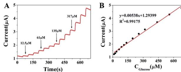
Fig. 4 (A) Amperometric response of Cu<sup>2+</sup>-Cu<sup>+</sup>/biochar/Au/GCE to the successive addition of glucose and (B) the corresponding calibration curve.
