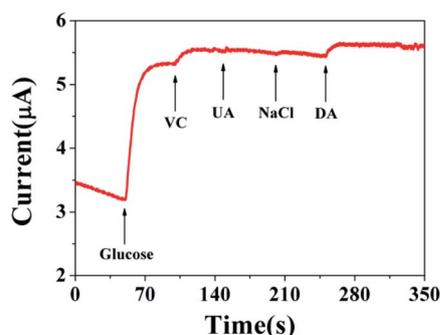
Fig. 5 Amperometric response curve of Cu<sup>2+</sup>–Cu<sup>+</sup>/biochar/Au/GCE obtained in the presence of 0.1 M NaOH at +0.6 V with continuous stirring to the successive addition of 5 mM glucose, 0.025 mM VC, 0.025 mM UA, 0.1 mM NaCl and 0.025 mM DA.
