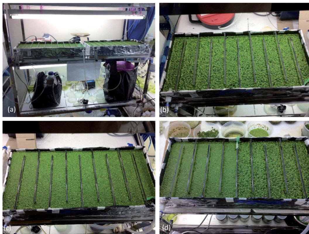
Fig. 1 (a) The setup of the raceway pond rig system in the laboratory. (b) The S. polyrhiza monoculture system. (c) The Lemna sp. monoculture system. (d) The S. polyrhiza + Lemna sp. polyculture system.
