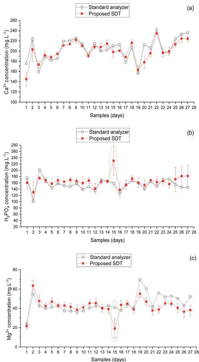
Fig. 9 Comparison between predicted ion concentrations of the smart diagnostic tool and standard analyzers. (a)  $\text{Ca}^{2+}$ , (b)  $\text{H}_2\text{PO}_4^-$ , and (c)  $\text{Mg}^{2+}$ . Error bars are three replicates' standard deviations.
