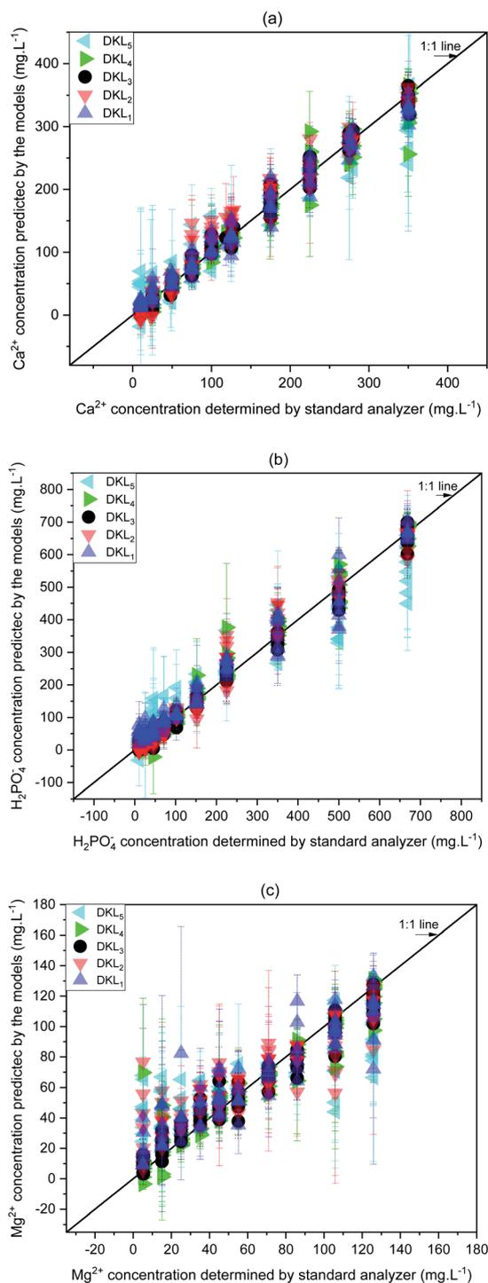
Fig. 6 Relationships between predicted ion concentrations of the DKL model and standard analyzers. (a) Ca<sup>2+</sup>, (b) H<sub>2</sub>PO<sub>4</sub><sup>-</sup>, and (c) Mg<sup>2+</sup>. Error bars are three replicates' standard deviations.
