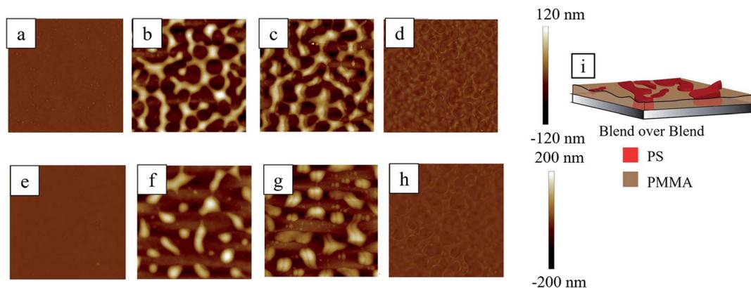
Fig. 7 AFM scans of  $20\ \mu\text{m} \times 20\ \mu\text{m}$  for blend over  $\sim 23\ \text{nm}$  blend after (a) spin coating (b) after RTA (c) acetic acid treatment and (d) cyclohexane treatment. Similarly, AFM scans of  $20\ \mu\text{m} \times 20\ \mu\text{m}$  for blend over  $\sim 53\ \text{nm}$  blend after (e) spin coating (f) RTA (g) acetic acid treatment and (h) cyclohexane treatment. A schematic of the morphology of PS/PMMA blend over blend after RTA is shown in (i).
