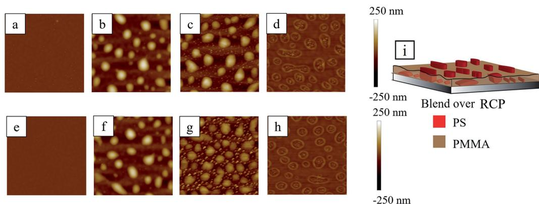
Fig. 8 AFM scans of  $20\ \mu\text{m} \times 20\ \mu\text{m}$  for blend over  $\sim 22\ \text{nm}$  RCP after (a) spin coating (b) RTA (c) acetic acid treatment and (d) cyclohexane treatment. Similarly, AFM scans of  $20\ \mu\text{m} \times 20\ \mu\text{m}$  for blend over  $\sim 49\ \text{nm}$  RCP after (e) spin coating (f) RTA (g) acetic acid treatment and (h) cyclohexane treatment. A macroscopic schematic of PS/PMMA blend over RCP after RTA is shown in (i).
