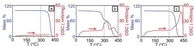
Fig. 3 TGA (blue line) and DSC (red line) for (a) PS (b) PMMA and (c) random PS-*r*-PMMA.
