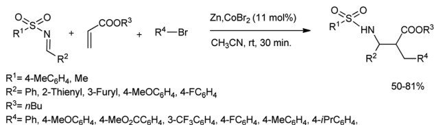
Scheme 31 Zinc-mediated Mannich reaction for the preparation of α,β-disubstituted N -sulfonyl β-amino esters.
