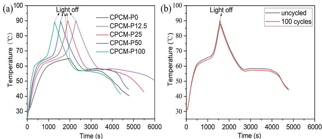
Fig. 11 Temperature–time curves of CPCMs under light irradiation at  $250 \text{ mW cm}^{-2}$ : (a) CPCMs, (b) CPCMs-P50 after 100 light on and off cycles.
