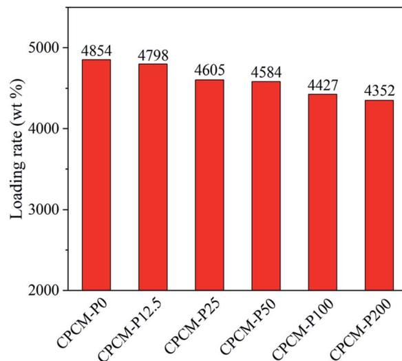
Fig. 4 Loading rates of *n*-octacosane for CPCMs.
