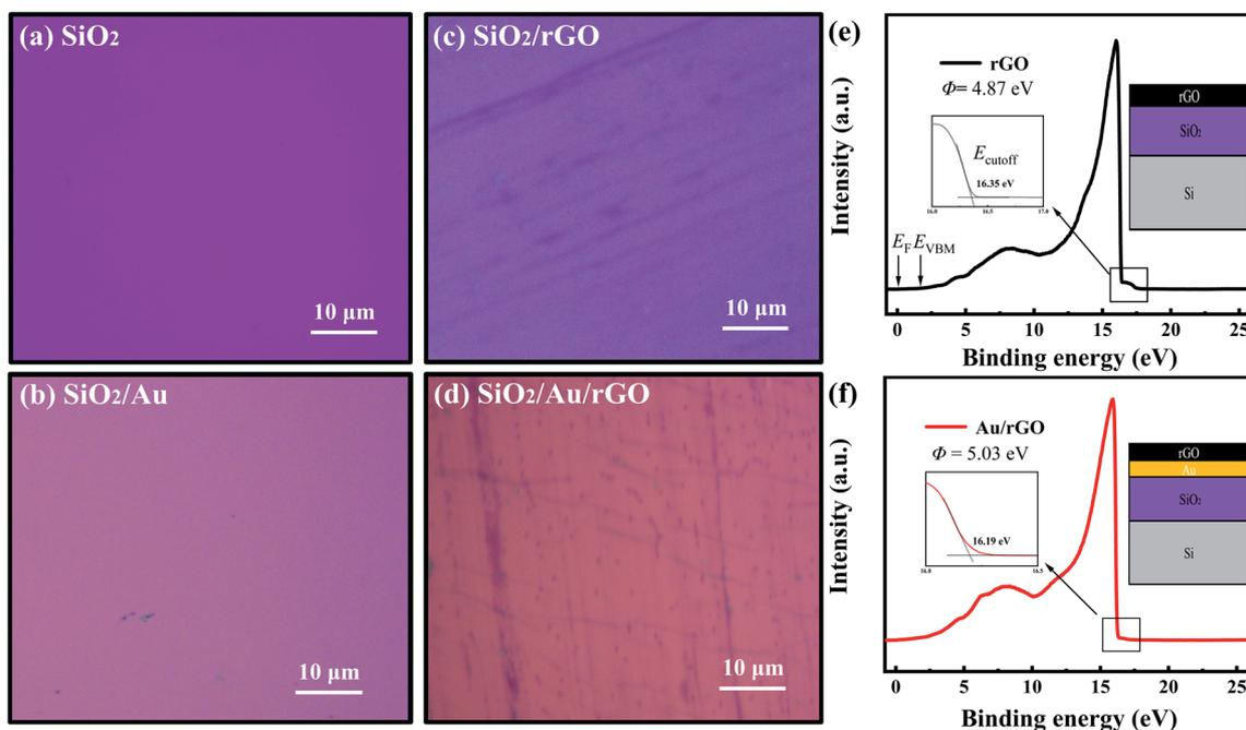
Fig. 5 Optical images of (a) Si/SiO<sub>2</sub> substrate, (b) Si/SiO<sub>2</sub>/Au substrate, (c) Si/SiO<sub>2</sub>/rGO, and (d) Si/SiO<sub>2</sub>/Au/rGO, and the UPS spectrum of (e) rGO and (f) Au/rGO.
