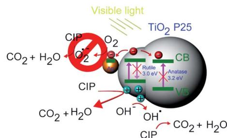
Scheme 2 Photocatalytic mechanism scheme of Ag-TiO<sub>2</sub> NPs under visible light.
