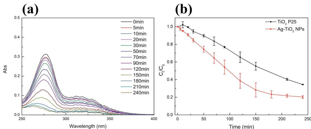
Fig. 6 (a) Representative variations of the absorption spectrum of NFX ( $3 \text{ mg L}^{-1}$ ,  $\text{pH} = 3$ ) under visible light irradiation by using Ag-TiO<sub>2</sub> NPs ( $300 \text{ mg L}^{-1}$ ); (b) time-dependent concentration of NFX solution upon exposure to visible light in the presence of TiO<sub>2</sub> P25 ( $300 \text{ mg L}^{-1}$ , black squares) and Ag-TiO<sub>2</sub> NPs ( $300 \text{ mg L}^{-1}$ , red circles); reported values are the mean of 3 replicates.
