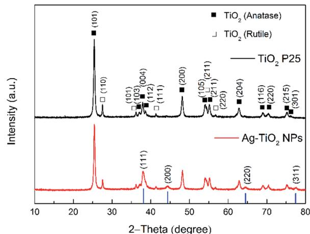
Fig. 1 Powder XRD patterns of TiO<sub>2</sub> P25 and Ag–TiO<sub>2</sub> NPs. The blue lines represent the diffraction peaks positions for the typical Ag XRD pattern (JCPDS no. 87-0717).
