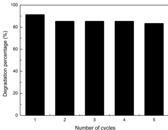
Fig. 7 Five photocatalytic degradation reactions of fresh CIP solution ( $3 \text{ mg L}^{-1}$ ,  $\text{pH} = 3$ ) with reused (for up to 5 cycles) Ag-TiO<sub>2</sub> NPs ( $300 \text{ mg L}^{-1}$ ) under visible light irradiation.
