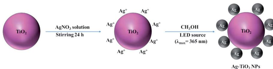
Scheme 1 Synthetic route for the preparation of Ag–TiO<sub>2</sub> NPs.
