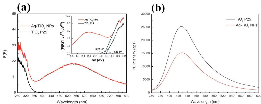
Fig. 4 (a) UV-Vis absorption spectra of TiO<sub>2</sub> P25 and Ag-TiO<sub>2</sub> NPs with the inset of Tauc plot and (b) PL spectra of TiO<sub>2</sub> P25 and Ag-TiO<sub>2</sub> NPs.
