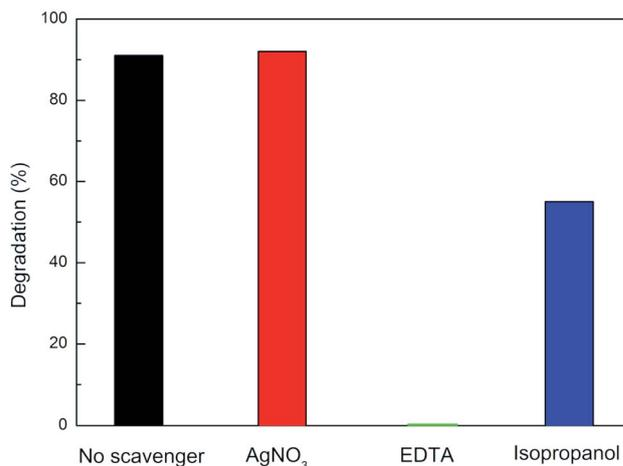
Fig. 8 Visible-light photocatalytic degradation percentage of CIP ( $3 \text{ mg L}^{-1}$ ,  $\text{pH} = 3$ ) in the presence of only Ag-TiO<sub>2</sub> NPs ( $300 \text{ mg L}^{-1}$ , in black) or of both Ag-TiO<sub>2</sub> NPs ( $300 \text{ mg L}^{-1}$ ) and the scavengers AgNO<sub>3</sub> (in red), EDTA (in green) or isopropanol (in blue).
