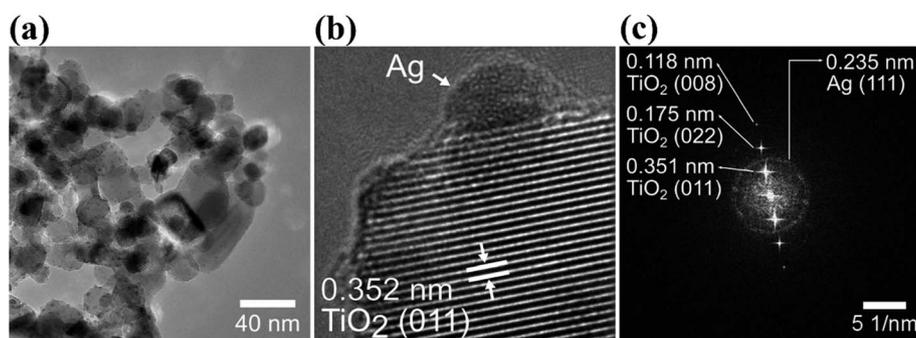
Fig. 3 HRTEM images at low magnification (a) and high magnification (b) of Ag-TiO<sub>2</sub> NPs; (c) SAED (selected area electron diffraction) pattern of Ag-TiO<sub>2</sub> NPs.
