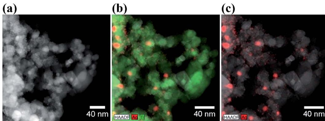
Fig. 2 (a) HRTEM image of Ag-TiO<sub>2</sub> NPs; (b) EDS map of Ag-TiO<sub>2</sub> NPs with Ag (red) and Ti (green) atomic distribution; (c) EDS map of Ag-TiO<sub>2</sub> NPs with Ag atomic distribution (in red).
