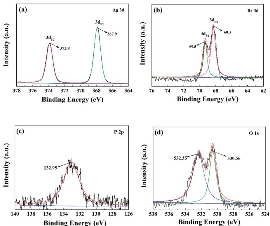
Fig. 3 XPS spectra of (a) Ag 3d, (b) Br 3d, (c) P 2p and (d) O 1s of the ABAP-48% composites.
