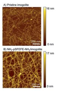
Fig. 4 SFM image of (A) pristine imagolite and (B)  $NH_2$ -pSFEFE- $NH_2$ / imagolite hybrid on Si wafer substrate.
