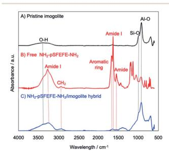
Fig. 2 ATR-FTIR spectra of (A) pristine imogolite, (B) free NH<sub>2</sub>-pSFEFE-NH<sub>2</sub>, (C) NH<sub>2</sub>-pSFEFE-NH<sub>2</sub>/imogolite hybrid.
