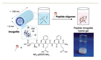
Fig. 1 Schematic diagram of hybrid gel preparation and image of the hybrid hydrogel (NH $_2$ -pSFEFE-NH $_2$ /imagolite hybrid (0.27 mg mL $^{-1}$ )).
