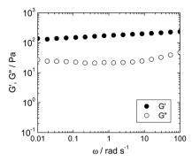
Fig. 3 Angular frequency ( $\omega$ ) dependence of storage modulus (G', filled circle) and loss modulus (G'', open circle) of NH<sub>2</sub>-pSFEFE-NH<sub>2</sub>/ imagolite hybrid (0.3 mg mL<sup>-1</sup>) at 25 °C.
