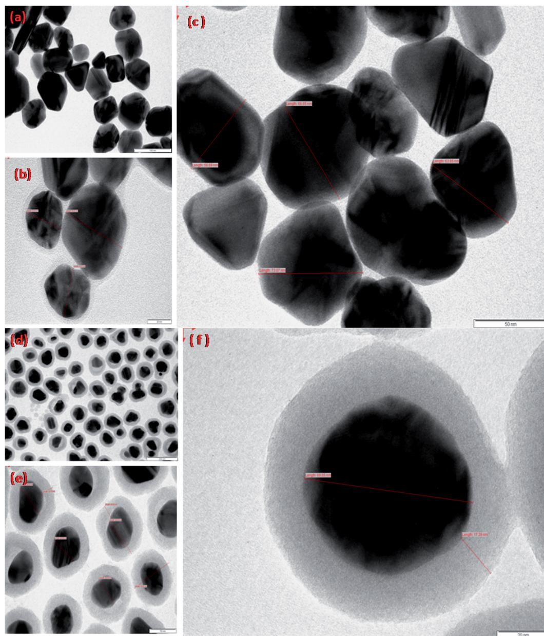
Fig. 2 TEM images of the prepared (a)–(c) Ag nanoparticles and (d)–(f) Ag@SiO<sub>2</sub> nanoparticles shown in the TEM images at different magnifications. As one can see, the Ag nanoparticles have a spherical shape with the average size of 50 nm, while the TEM images of Ag@SiO<sub>2</sub> nanoparticles show uniform, clean, and distinct coating of silica on the surface of the Ag nanoparticles; the Ag@SiO<sub>2</sub> nanoparticles have an average size of 80 nm.
