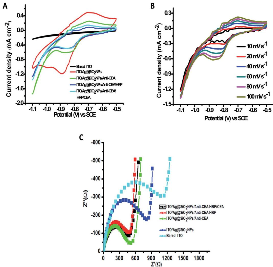
Fig. 6 (A) CV of the stepwise immunosensor fabrication process at a scan rate of  $60 \text{ mV s}^{-1}$  using  $0.1 \text{ M}$  pH  $6.0$  PBS buffer solution, which contains  $\text{Na}_2\text{HPO}_4$  and  $\text{NaH}_2\text{PO}_4$ . (B) CV of the fabricated immunosensor at different scan rates. (C) EIS related to the various steps elaborated in the manufacturing process.
