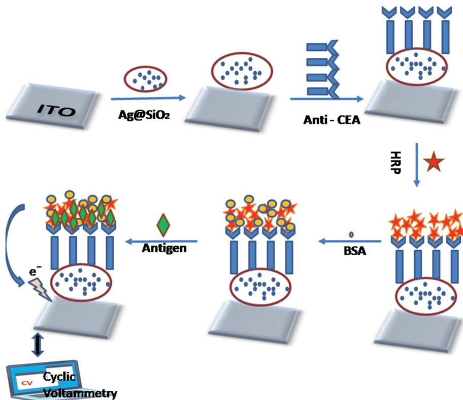
Fig. 4 Process flow for disposable electrochemical immunosensor fabrication.
