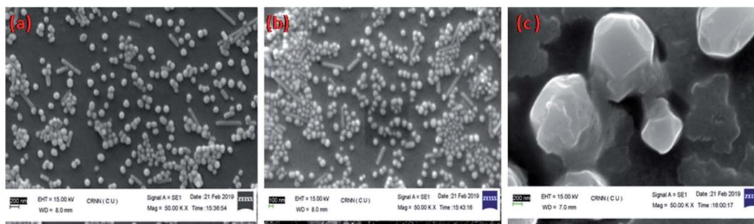
Fig. 5 SEM of (a) Ag@SiO<sub>2</sub> nanoparticles on ITO film, (b) CEA/HRP/anti-CEA/Ag@SiO<sub>2</sub> NPs at Mag 1.00 hX, (c) CEA/HRP/anti-CEA/Ag@SiO<sub>2</sub> NPs at Mag 5.00 kX.
