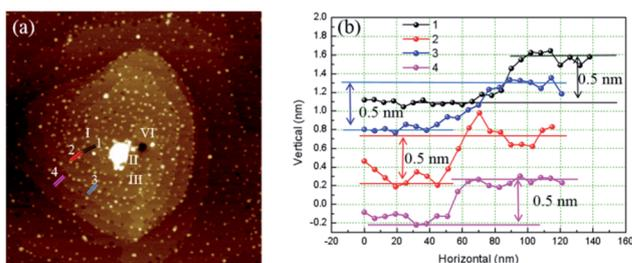
Fig. 4 (a) AFM image of hillocks with  $b_\perp = 4h$  (b) cross section along different colors segments.
