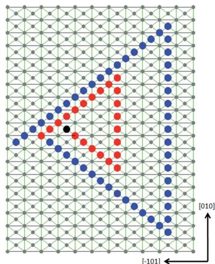
Fig. 10 The projection view of the growth spiral on (101) face along the  $[110]$  direction. Two growth loops are presented with a moving speed of 1, 2, 6 layers for each step each time. The black dots represent the terminal of screw dislocation. Red dots and blue dots represent the edge of two terraces (steps) has grown on the surface.
