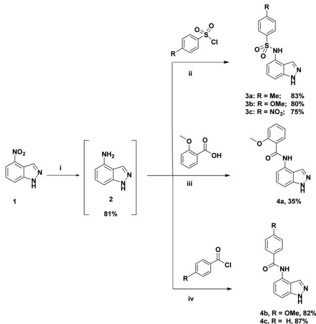
**Scheme 1** Reagents and conditions for the synthesis of **3a–c** and **4a–c**. Reaction conditions. (i) Fe/NH<sub>4</sub>Cl (6/10 equiv.), EtOH, rt for 3 h, 81%; (ii) ArSO<sub>2</sub>Cl (1 equiv.), pyridine, 24 h, 75–83%; (iii) *o*-methoxy benzoic acid (1 equiv.), TBTU (1 equiv.), DIPEA (3 equiv.), DMF, rt for 16 h, 35%. (iv) *p*-methoxy benzoyl chloride (1.1 equiv.), DIPEA (2 equiv.), DCM, 0 °C–rt for 18 h, 82%.
