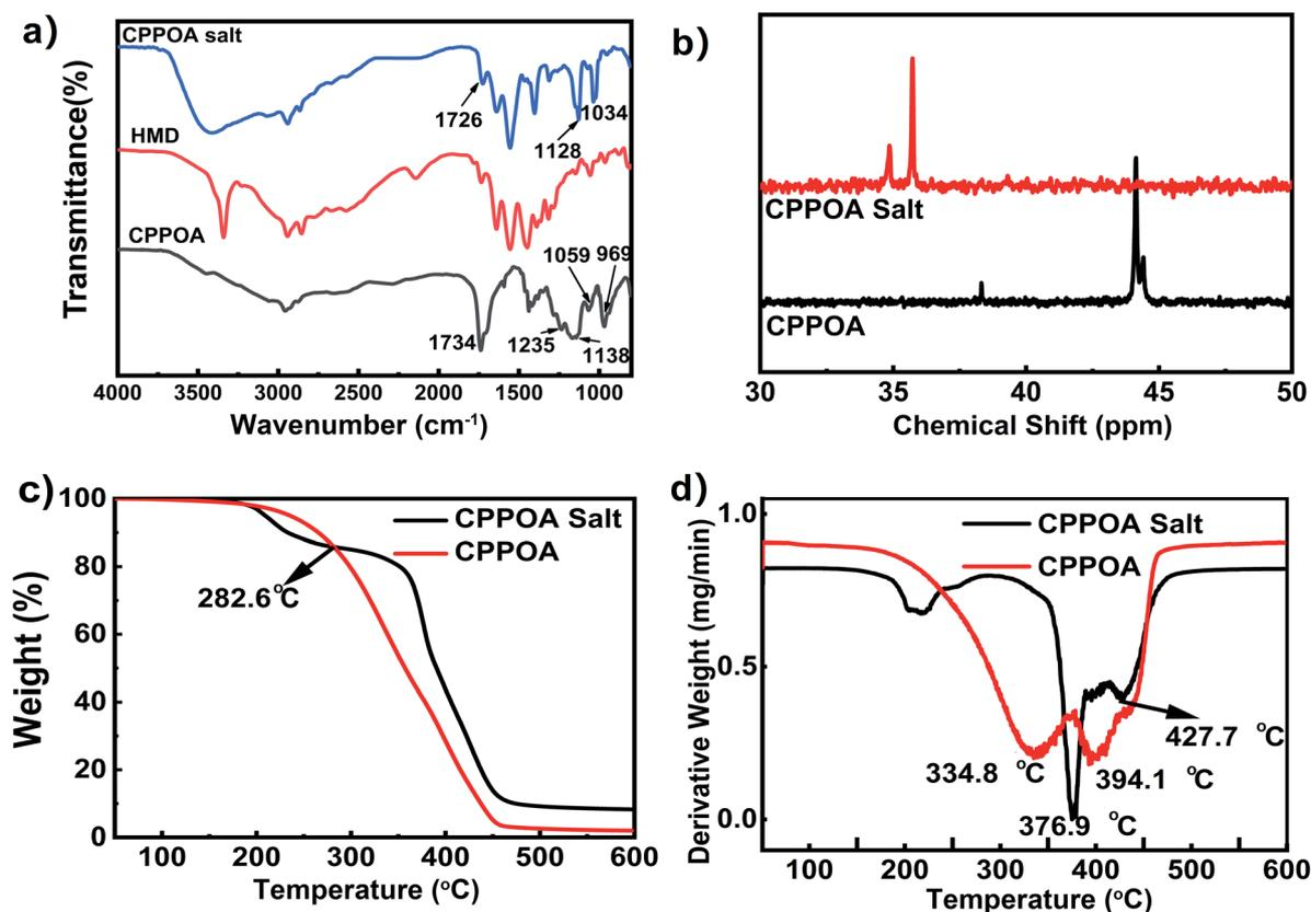
Fig. 3 Structural characterization and thermal analysis of flame-retardants: (a) FTIR spectra of CPPOA, HMD, and CPPOA salt; (b) <sup>31</sup>P-NMR spectra of CPPOA and CPPOA salt; (c) TGA and (d) DTG curves of CPPOA and CPPOA salt.
