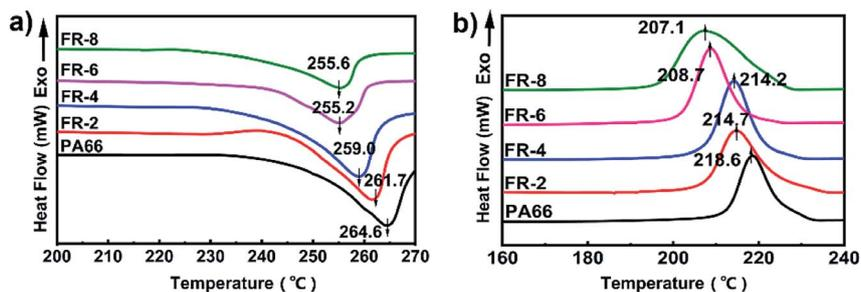
Fig. 5 DSC curves of PA66 and FRPA66 (a) heating (b) cooling.
