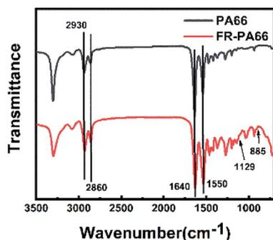
Fig. 10 Infrared spectra of carbon residues of PA66 and FRPA66.
