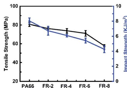
Fig. 11 Mechanical properties of PA66 and FRPA66.
