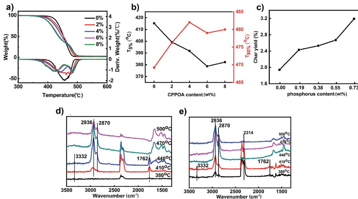
Fig. 7 (a) TGA-DTG curves of PA66 and FRPA66; (b) plots for  $T_{5\%}$  and  $T_{end}$  values of FRPA66 and FRPA66; (c) the relationship between residual char content and phosphorus content; IR spectra of (d) pure PA66 at different pyrolysis temperatures; (e) 6 wt% FRPA66 at different pyrolysis temperatures.
