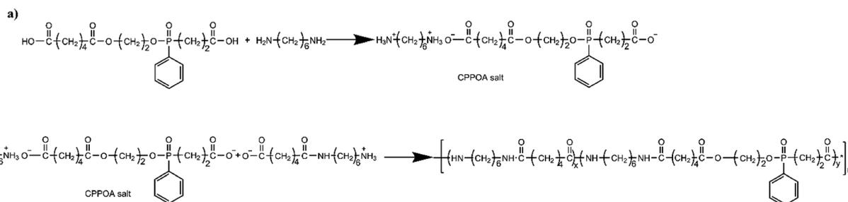
Fig. 2 Route for synthesis of (a) CPPOA salt and (b) FRPA66.
