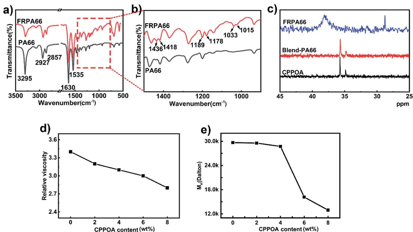
Fig. 4 (a) FTIR spectra of PA66 and FRPA66. (b) Enlarged view of  $900\text{--}1500\text{ cm}^{-1}$  spectral range. (c)  $^{31}\text{P}$ -NMR spectra of CPPOA salt, blend-PA66, and FRPA66. (d) Relative viscosities of PA66 and FRPA66. (e) Number average molecular weight ( $M_n$ ) of PA66 and FRPA66.
