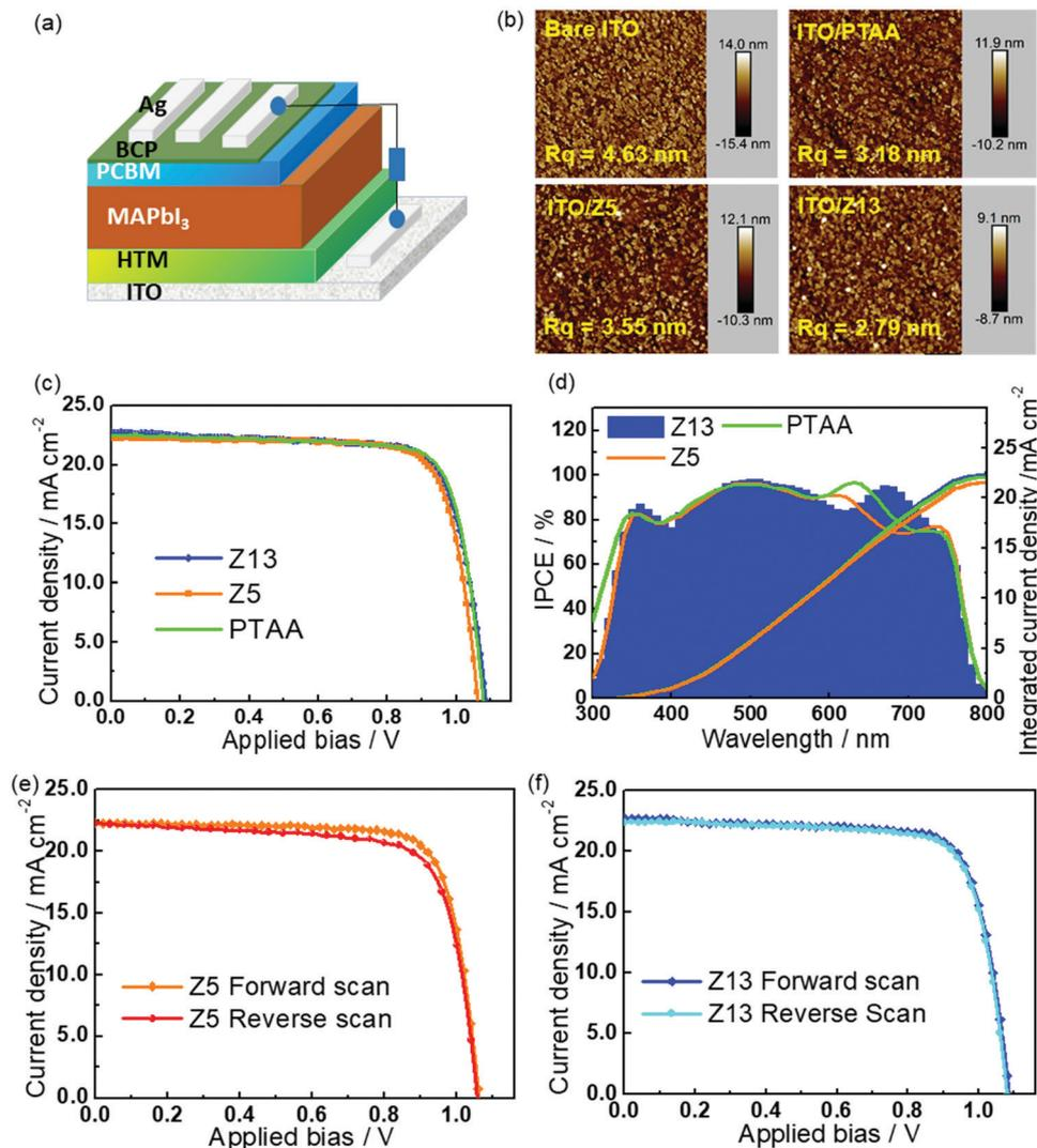
Fig. 4 (a) Device architecture of p-i-n i-PSCs; (b) atomic force microscopy images; (c)  $J$ - $V$  curves of the i-PSCs in the forward scanning direction under AM 1.5G,  $100 \text{ mW cm}^{-2}$  illumination; and (d) EQE spectra of the corresponding i-PSCs;  $J$ - $V$  curves measured with forward and reverse scanning for Z5 (e) and Z13 (f), respectively.
