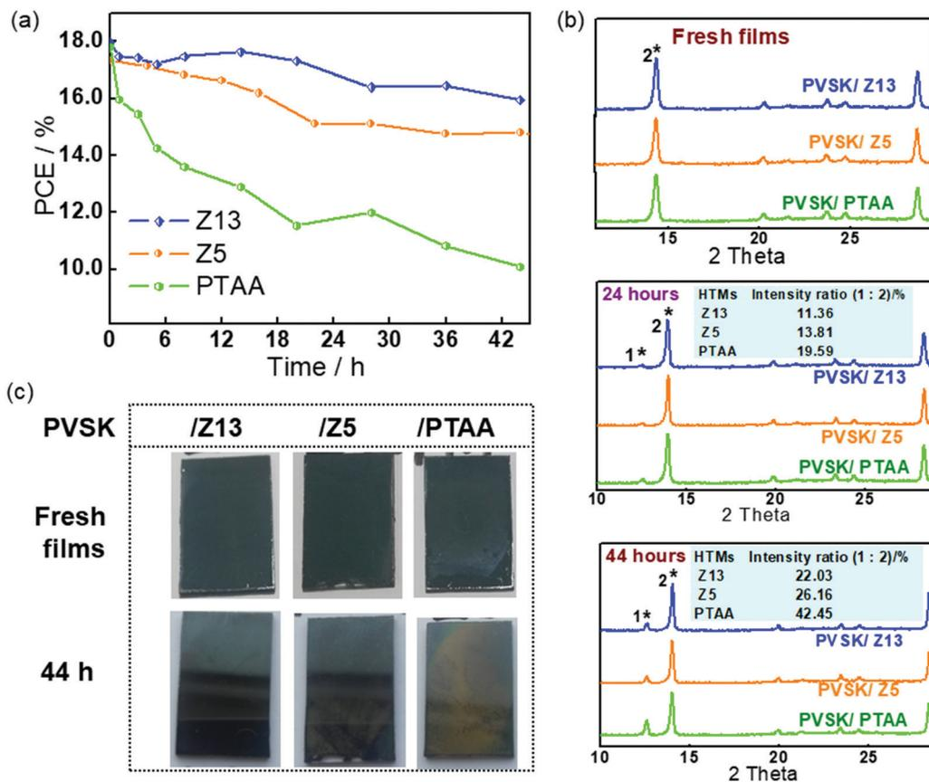
Fig. 6 Stability analysis. (a) PCE evolution of unencapsulated i-PSCs heated at 85 °C under a N<sub>2</sub> atmosphere (30% relative humidity); (b) XRD pattern evolution of i-PSCs with different HTMs; and (c) perovskite (PVSK) film-degradation evolution during heating.
