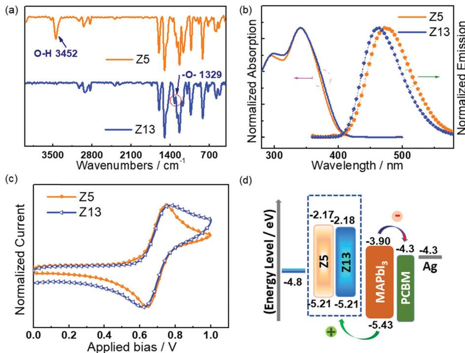
Fig. 2 (a) FT-IR spectra of Z13 and Z5; (b) UV-vis absorption and photoluminescence spectra of HTMs in  $\text{CH}_2\text{Cl}_2$ ; (c) cyclic voltammetry curves; and (d) energy levels in i-PSCs.
