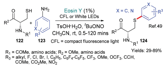
Scheme 31 Biocompatible conditions for the arylation of cysteines 122 \rightarrow 124 in either batch or flow.
