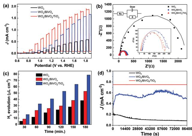
**Fig. 6** Photoelectrochemical performance of  $\text{WO}_3$ ,  $\text{WO}_3/\text{BiVO}_4$ , and  $\text{WO}_3/\text{BiVO}_4/\text{TiO}_2$  photoelectrodes: (a) Linear sweep voltammetry curves, (b) Nyquist plots and equivalent circuit, (c) plot of  $\text{H}_2$  evolution as a function of time, and (d) chronoamperometric current density–voltage ( $J$ – $T$ ) curves.
