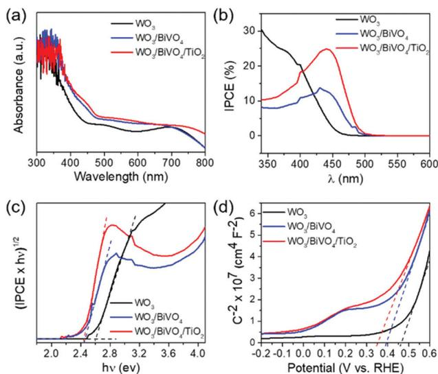
Fig. 5 Optoelectronic characterization of (a) UV-vis absorption spectra, (b) IPCE spectra, (c)  $(\text{IPCE} \cdot h\nu)^{1/2}$  *vs.*  $h\nu$  plots, and (d) Mott-Schottky plots of  $\text{WO}_3$ ,  $\text{WO}_3/\text{BiVO}_4$ , and  $\text{WO}_3/\text{BiVO}_4/\text{TiO}_2$  photoelectrodes.
