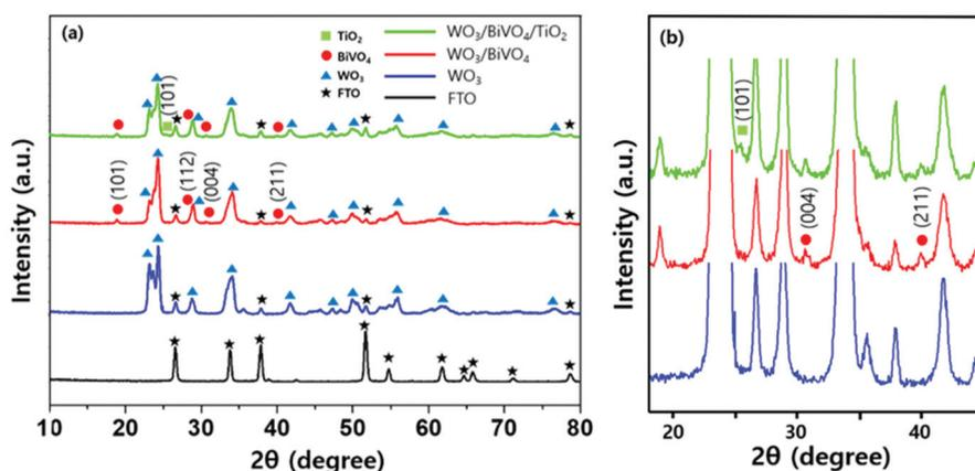
Fig. 2 XRD patterns of (a) FTO,  $\text{WO}_3$ ,  $\text{WO}_3/\text{BiVO}_4$ , and  $\text{WO}_3/\text{BiVO}_4/\text{TiO}_2$  samples and (b) the corresponding magnified view.
