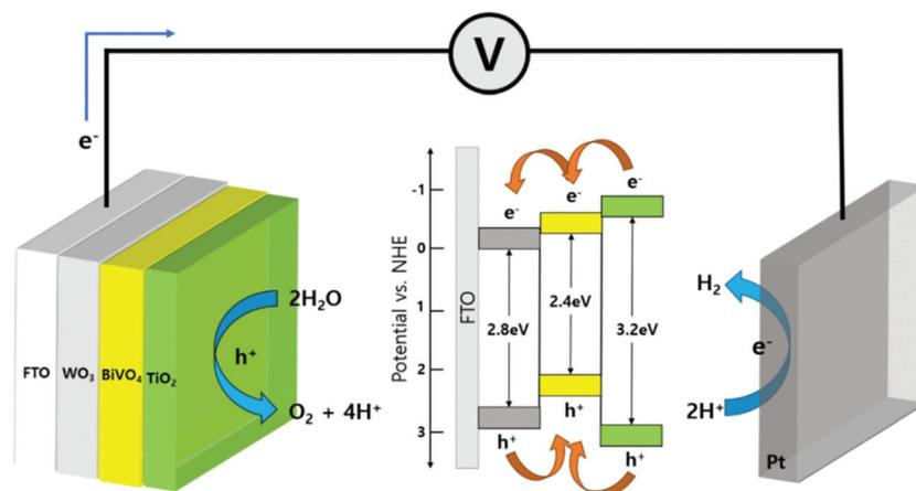
Fig. 7 Electron transfer mechanism of a  $\text{WO}_3/\text{BiVO}_4/\text{TiO}_2$  photoelectrode.
