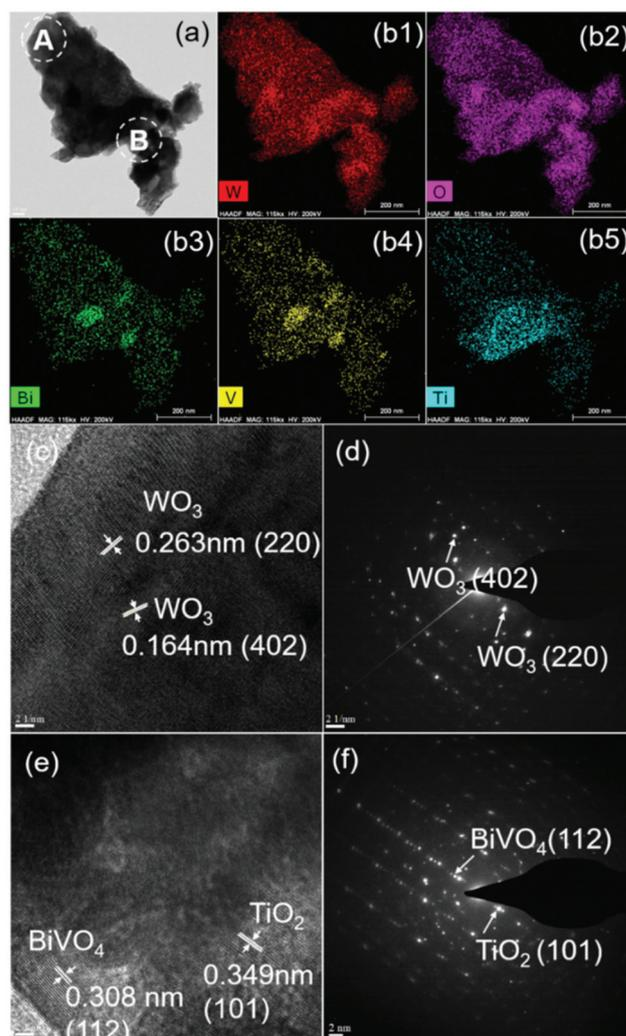
Fig. 3 (a) TEM image recorded in the HADDF mode of  $\text{WO}_3/\text{BiVO}_4/\text{TiO}_2$ ; (b1–b5) corresponding elemental analysis by EDS mapping of W, O, Bi, V, and Ti levels; (c) HR-TEM images of  $\text{WO}_3/\text{BiVO}_4/\text{TiO}_2$  for areas marked A in 3(a); (d) corresponding SAED pattern; (e) HR-TEM images of  $\text{WO}_3/\text{BiVO}_4/\text{TiO}_2$  for areas marked B in 3(a); and (f) corresponding SAED pattern.
