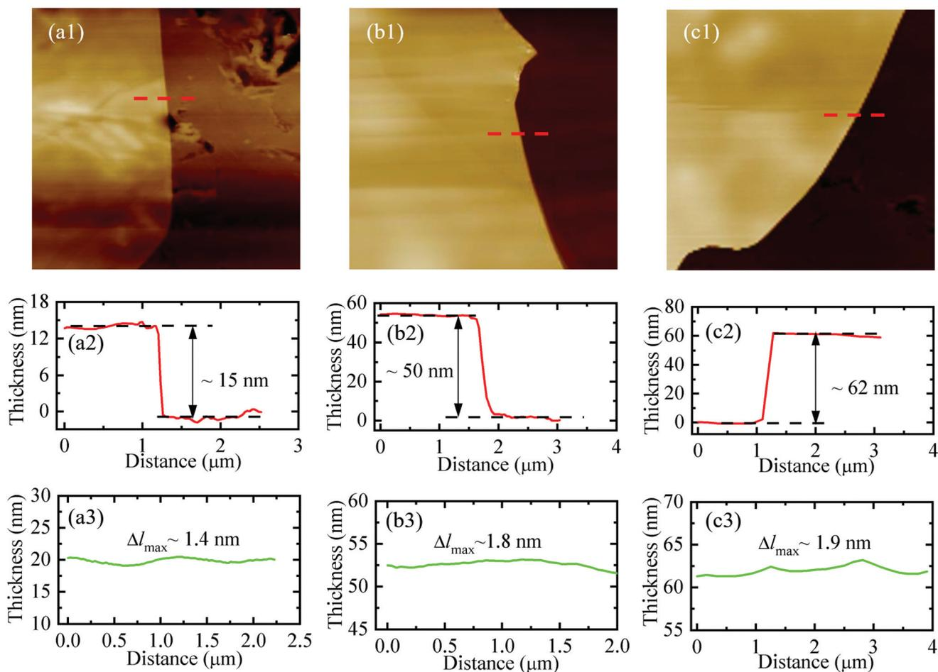
**Fig. 2** AFM measurement results of three suspended MoSe<sub>2</sub> samples. (a1)–(c1) AFM images of three samples. (a2)–(c2) Thickness profiles corresponding to the red dashed line in figure (a1)–(c1). (a3)–(c3) Thickness profiles indicate the roughness of the measured area of three samples.
