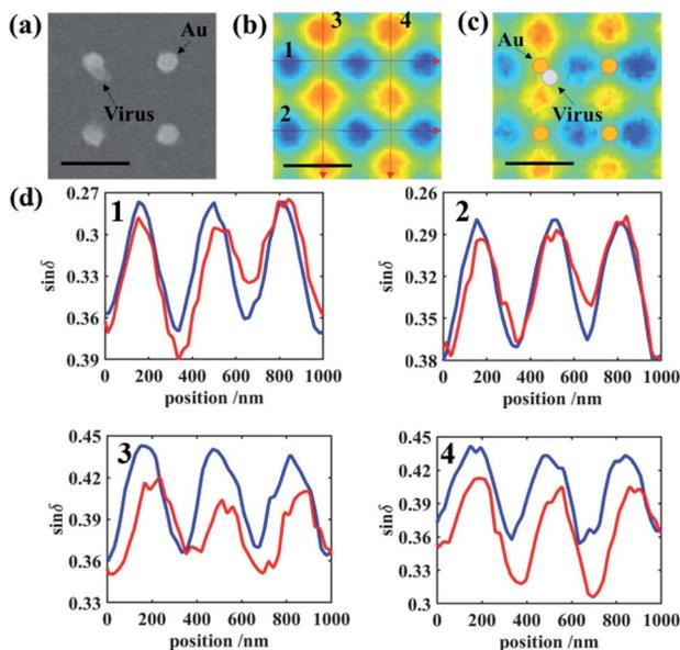
Fig. 5 (a) SEM image of a four-quadrant sensor with a virus, (b)  $\sin \delta$  image of the four-quadrant sensor before deposition, (c)  $\sin \delta$  image of the four-quadrant sensor after deposition, and the scale bar for (a)–(c) is 0.5  $\mu\text{m}$ , (d) four characteristic curves labeled in (b). Blue curves represent bare gold and red curves represent gold attached to the virus.
