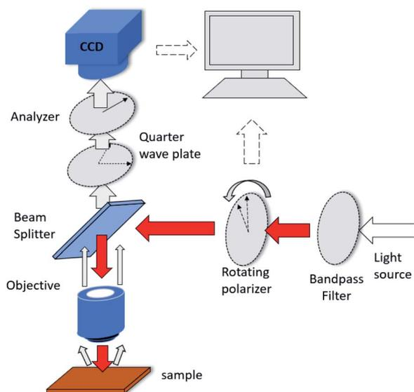
Fig. 2 Diagram of measurement using the PIMI system.
