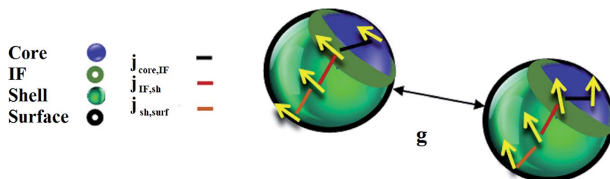
Fig. 1 Schematic representation of a system of dipolarly interacting core/shell nanoparticles. The nanoparticle architecture (soft/hard or hard/soft) defines the strength of the exchange intraparticle interactions ( J_{\text{core-IF}} , J_{\text{IF-shell}} , J_{\text{shell-surf}} ) between the four macro-spins ( S_{\text{core}} , S_{\text{IF}} , S_{\text{shell}} , S_{\text{surf}} ) for the core, shell, interface and surface regions respectively, in the mesoscopic model. Each spin also interacts with the spins of the neighbouring nanoparticles via dipolar interactions.
