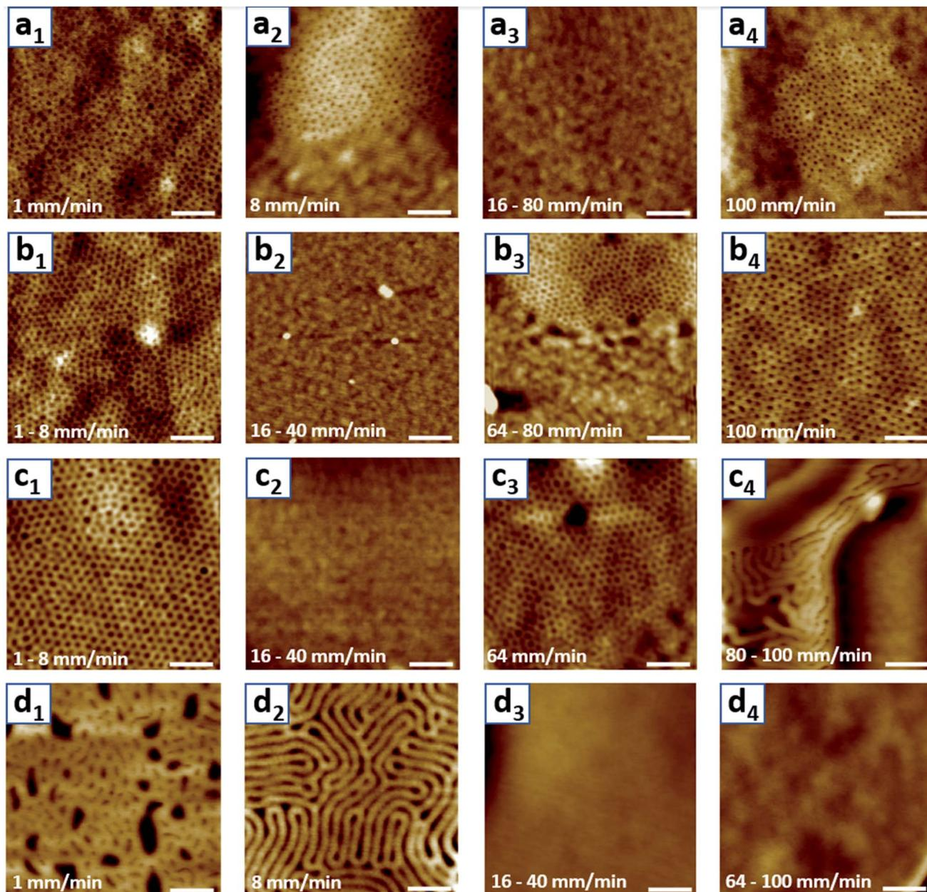
Fig. 1 Representative AFM height images of films dip-coated from  $10 \text{ mg ml}^{-1}$  PS-*b*-PEO solutions containing varying contents of water in THF: (a<sub>1</sub>–a<sub>4</sub>) V<sub>0</sub>, (b<sub>1</sub>–b<sub>4</sub>) V<sub>2</sub>, (c<sub>1</sub>–c<sub>4</sub>) V<sub>5</sub> and (d<sub>1</sub>–d<sub>4</sub>) V<sub>10</sub>. The white bar represents a scale of 200 nm.
