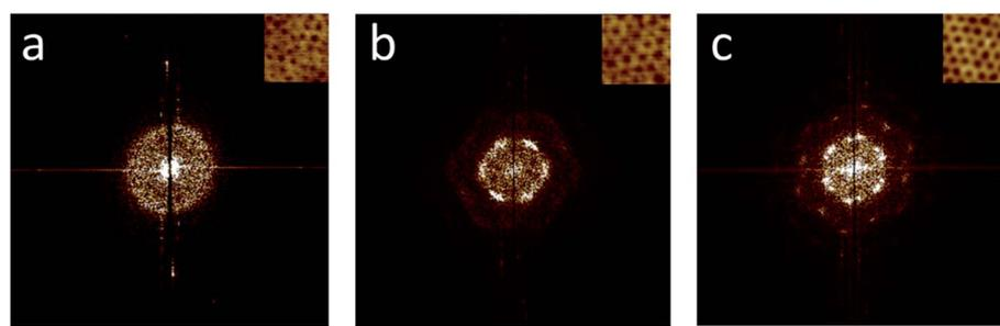
Fig. 4 Fast Fourier transform (FFT) of AFM images for the evaluation of the ordering of the cylinders formed from different solutions: (a)  $V_0$  (1, 8 and 100 mm  $\text{min}^{-1}$ ), (b)  $V_2$  (1–8, 64–80 and 100 mm  $\text{min}^{-1}$ ) and (c)  $V_5$  (1–8 and 64 mm  $\text{min}^{-1}$ ). The size of the inset AFM images is 200 × 200 nm.
