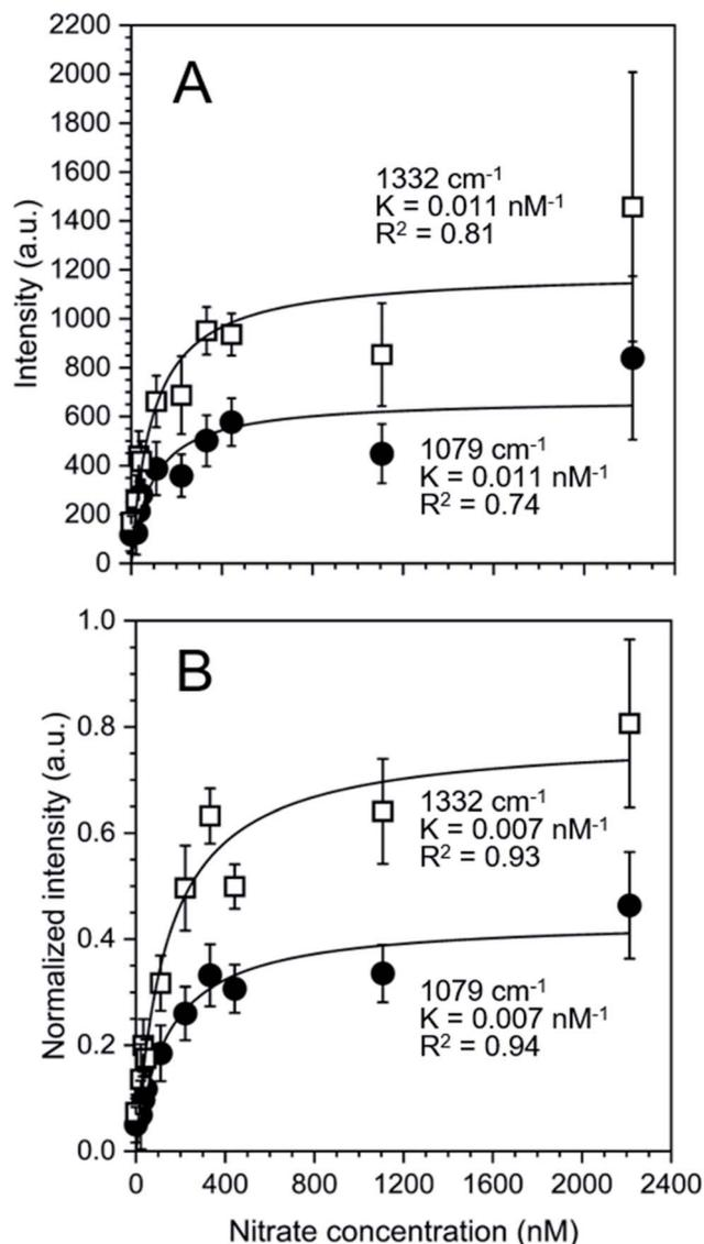
Fig. 4 (A) Intensity and (B) normalized intensity of the peaks at  $1079\text{ cm}^{-1}$  (closed circles ●) and  $1332\text{ cm}^{-1}$  (open squares □) as a function of nitrate concentration. Error bars represent the time-averaged standard deviation of the intensities at the specified wave-numbers. The solid lines show the fitted Langmuir adsorption model and the Langmuir constant  $K$  and the goodness of fit,  $R^2$ , are reported.
