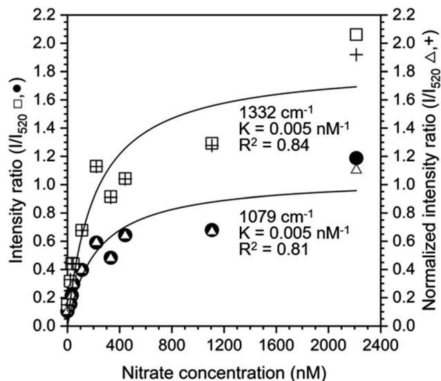
Fig. 5 Intensity and normalized intensity ratios ( $I/I_{520}$ ) based on the silicon peak at  $520\text{ cm}^{-1}$  and nitrate peaks at  $1079\text{ cm}^{-1}$  (closed circles ●, open triangles  $\Delta$ ) and  $1332\text{ cm}^{-1}$  (open squares □, plus signs +) as a function of nitrate concentration. The solid lines show the fitted Langmuir adsorption model and the Langmuir constant  $K$  and the goodness of fit,  $R^2$ , are reported.
